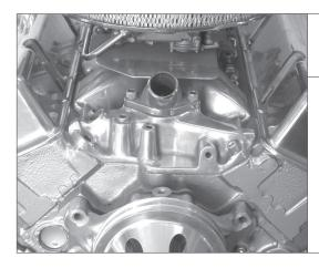
REMOVE the 2 upper water pump bolts.
