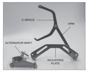
REMOVE the alternator bracket and set to the side, keeping the adjusting plate, C-Brace and arm together as shown in the photo.
