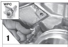
**INSTALL** the WPC (inset) by removing the top water pump bolt. Leave slightly loose.
