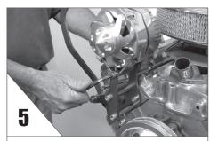
**INSTALL** the alternator to the bracket. **PLEASE** keep the 7/8" spacer between the alternator and back plate.
