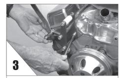
**INSTALL** the bracket to head and snug up. Pivot the adjusting arm out to the side for now.
