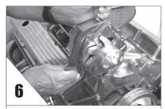
**SWING** the adjusting arm up and bolt it to the alternator.
