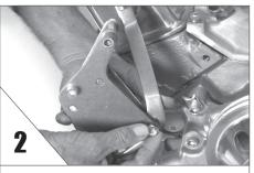
**REMOVE** the nut and plastic sleeve from bracket. Keep bolts and adjusting arm in place. Do not disasseble the bracket.
