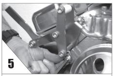
**PUSH** the WPC up to the lower spacer and tighten.
