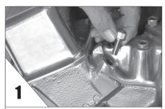
**REMOVE** the 1st intake manifold bolt.
