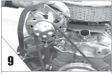
**ADJUST** belt for tension. **TIGHTEN** up all the bolts now and check for alignment.
