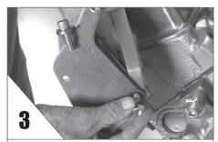
**REMOVE** the nut and plastic sleeve from bracket. Keep bolts and adjusting arm in place. Do not disasseble the bracket.
