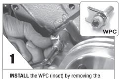
top water pump bolt. Leave slightly loose.
