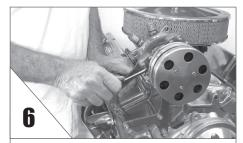
SWING the adjusting arm up and bolt it to the compressor with the two bolts. Snug the bolts only for now, not tight.
