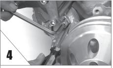
Using a FLATHEAD Screw Driver, LIFT the WPC up to the lower spacer and tighten.
