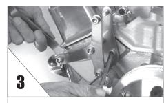
INSTALL the bracket to head and intake manifold and snug up. Pivot the adjusting arm out to the side for now.
