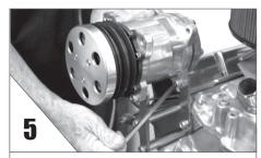
**INSTALL** the compressor to the bracket as shown abobe.
