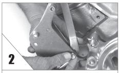
**REMOVE** the nut and plastic sleeve from bracket. Keep bolts and adjusting arm in place. Do not disassemble the bracket.
