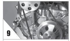
**ADJUST** belt for tension. **TIGHTEN** up all bolts now and check for proper alignment.
