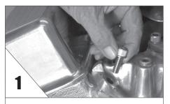
**REMOVE** the 1st intake manifold bolt.
