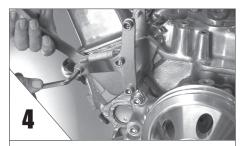
**INSTALL** the bracket to head and intake manifold and snug up. Pivot the adjusting arm out to the side for now.
