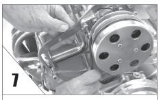
**SWING** the adjusting arm up and bolt it to the compressor with the two bolts. Snug the bolts only for now, not tight.
