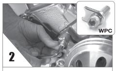
**INSTALL** the WPC (inset) by removing the top water pump bolt. Leave slightly loose.
