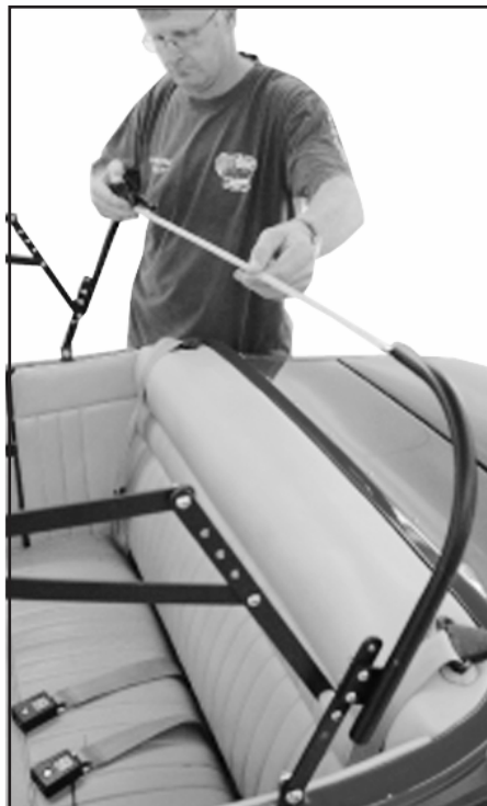
Above: Before undertaking the next step, make sure all the screws that hold the frame together are tightened firmly.
