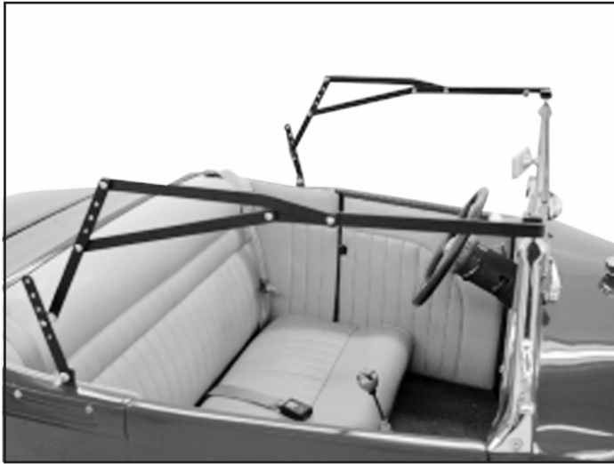
Above: With both sides mounted on the car car, the top is ready to be fitted with its wooden header panel.
