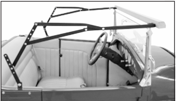
Left: Wood screws are used to secure the wooden header panel to the front of the brackets.
