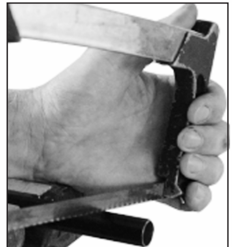
Below: A hacksaw is all that is needed to cut the straight section of cross bow to length. Measure twice, cut once.
