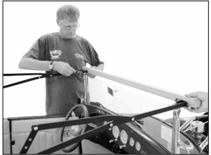
Above: The wooden header panel is held in place against the front edge of the windshield post mounts and the screw holes marked for pilot drilling.
