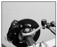
Ford spindle with tie rod ends
