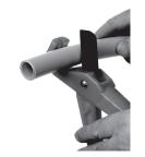
**1)** CUT the tubing square with the cutter, ROTATING wrist while cutting
