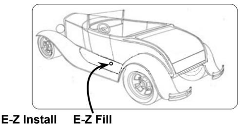
The E-Z Fill tanks bolt on with your running board brackets. After plumbing and wiring as per the instructions provided with your switchover valve:
