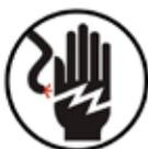
13. **DANGER!** The power unit used on this lift contains high voltage. Disconnect power at the receptacle before performing any electrical repairs. Secure plug so that it cannot be accidentally plugged in during service.
