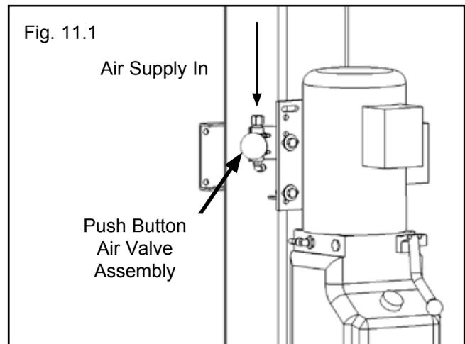
2. Route the air line that was left unconnected in Step 10 to the 90° Air Line Compression Fitting of the Push Button Air Valve Assembly. (See Fig 11.2)
