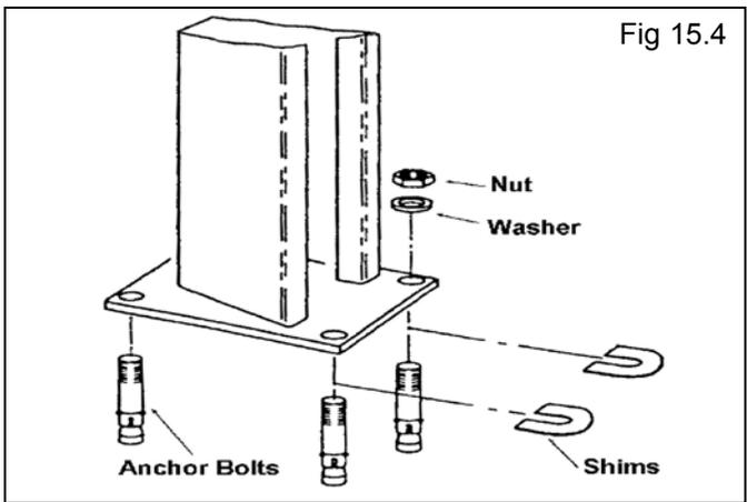
6. After any necessary shims are installed, tighten each nut 3-5 turns past hand tight. **IMPORTANT** - If anchor bolts do not hold when tightened to indicated amount, concrete must be replaced. Saw cut and remove 24" x 24" square area each column base then re-pour with reinforced 2500 PSI concrete to a depth of six inches minimum, keying new concrete under existing floor. (See Fig. 15.5)
