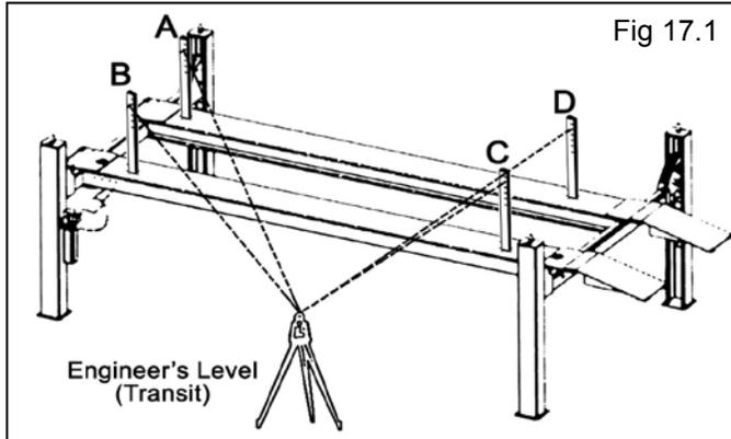
2. Follow the Level manufacturer's instructions for proper setup of the Level. Be sure it is adjusted level in all directions.
