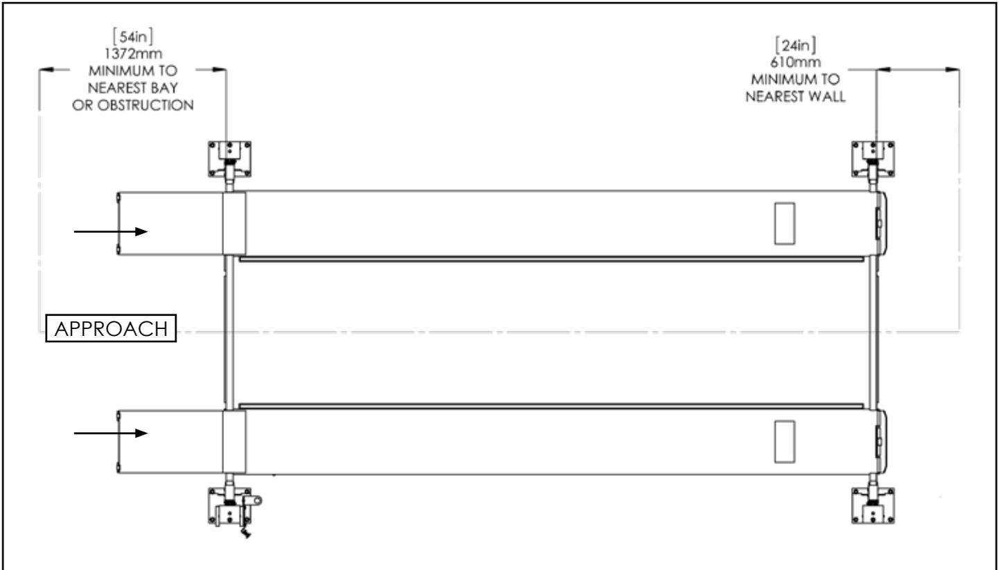
1. Lift Location: Use architects plan and Engineers automatic level (transit) when available to locate lift. The above shows clearances of a typical bay layout. Lift floor area should be level.
