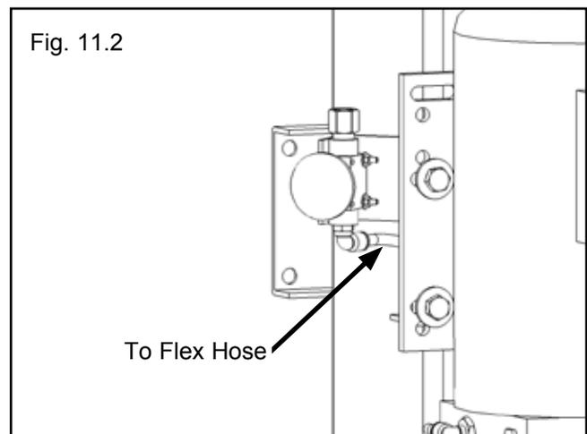
3. Once the air line has been connected with the Push Button Air Valve, cut the air lines to length by following the Safety Air Line Routing diagram located on Page 22 and connect female branch “tee” fittings where needed.
