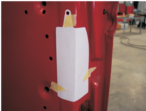
Fig. 3a Secure template with tape
