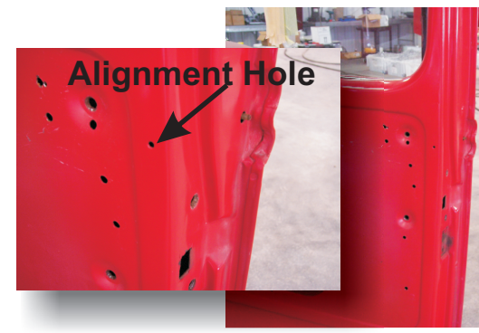
Fig. 3 Align template using existing hole
