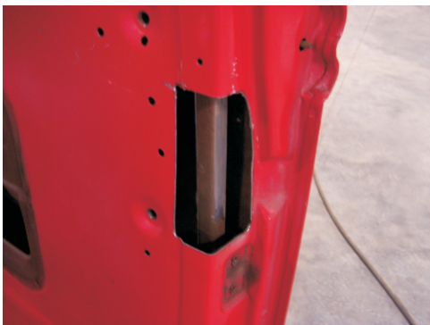
Fig. 5a Carefully cut hole for latch assembly
