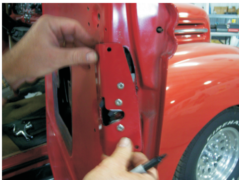
Fig. 6 Fit the latch assembly in place and mark mounting holes to be drilled. Remove latch and drill holes using a 1/4" drill bit.
