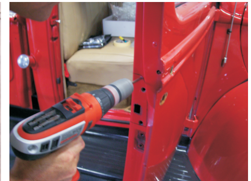
Fig. 5 Drill 1/4" holes in each corner
