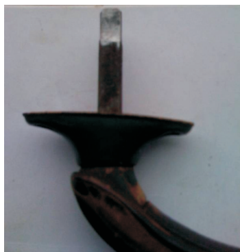
Fig. 2 File or sand shaft to size
