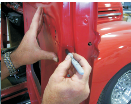
Fig. 6 Fit the latch assembly in place and mark mounting holes to be drilled. Remove latch and drill holes using a 1/4" drill bit.
