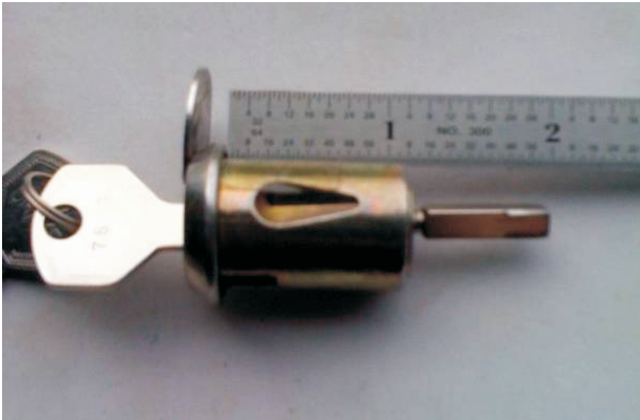
Fig. 9 Measure from the bottom of the lock cylinder bezel 1 3/4" and cut lock cylinder shaft. If you are installing lock cylinders in the drivers side it will need to be cut at 1 7/8". It is necessary to purchase our installation kit for installing lock cylinders in your drivers side door.
