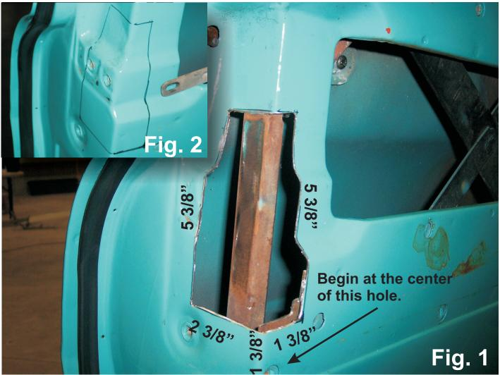
Starting at the center of the mounting hole shown in the image measure up 1 3/8". Mark a point with a pen or marker. Measure 1 3/8" starting at the corner of the door moving toward the center of the door. Mark a point. Measure straight up 5 3/8" and mark a point. Starting at your original point on the corner of the door measure 2 3/8" moving toward the outside of the door. Mark a point. Measure straight up 5 3/8" and mark a point. Connect your points and you have your cut line.
