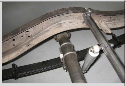
As pictured above, draw a line 28-1/8" in front of the rear bed bolt hole on top of each rail. Center the shock cross member on the top of the rails and mark the hole centers on the lines just drawn. Drill holes through the rail perpendicular to the surface. Drill only the top of the rails and then set the cross member in place and use a transfer punch to mark the hole centers on the bottom of the rail.
