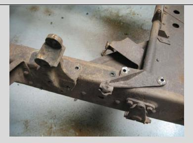
Start by removing the front stock spring hangers and e-brake cable bracket. To remove the rivets holding the brackets, grind the rivet heads flush. Center punch the rivet and drill through using progressively larger drills up to a 5/16" drill. The rivet should be relatively easy to punch out. If it is not, then continue drilling with a 3/8" drill. Take care not to drill the original rivet holes larger or off center, as you will be locating your now parts with these holes.
