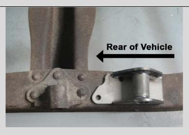
Remove the stock rear shackle bracket rivets in the same manner as the front spring hanger bracket rivets. The shackle brackets are positioned on the rails with the welded side on the inside of the rail. Line up the brackets with the holes of the original brackets. It may be necessary to align-drill a couple of these holes. Use three 3/8-16 x 1-1/4 bolts, nuts, and one washer under each nut to fasten each bracket. The square front edge of the bracket faces to the front of the vehicle.
