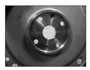
Install flywheel on engine. Again, make sure the mating surfaces of the flywheel and crank hub are clean and free of nicks or burrs. Look closely at the flywheel. Note that there are 4 holes in the center hub that are drilled through and 2 additional holes 180° apart. Align the 2 holes with the crankshaft dowel pins and use the 4 included bolts to secure the flywheel to the crank.
