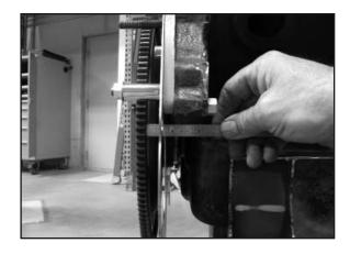
The final dimension check is for the starter drive engagement depth. With the flywheel installed and the block plate secured to the adapter, measure from the starter mating surface (the forward side of the block plate) to the front of the ring gear teeth. This dimension must be greater than .625 (5/8").
