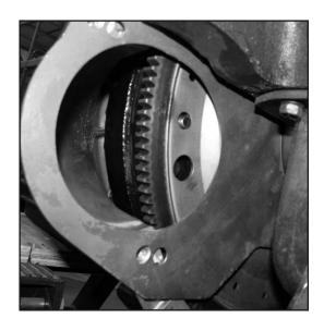
Rotate the flywheel so that one of the torque converter stud holes and the drain plug hole are lined up with the starter cutout in the block plate. Rotate torque converter on trans to place the drain plug and stud in the starter pocket area. Position the trans on the studs of the adapter plate and install 2 nuts, but do not tighten. Support the trans with a jack, do not allow it to hang on the studs.
