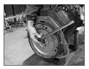
The hub fits the crank tightly and you will have to pull the flywheel on using the bolts. Do not use a hammer to seat the flywheel as you could damage the crank main bearings. Snug the bolts down in an alternating pattern until the flywheel is completely seated. Torque bolts to 50 ft. lb.
