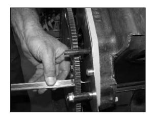
In some situations, like when using the old style case and small 157 tooth flywheel, the converter clearance dimension may exceed the stacking limit. In this case, remove the block plate and go through the dimensional checks again. In some very rare applications if the dimension is less than minimum it may be necessary to install 2 block plates.
