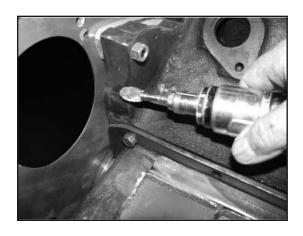
With the block plate in position, temporarily install the transmission on the engine without the flywheel. Hold the starter in position and note where it contacts the engine block. Using a die grinder or 4" angle grinder, grind 1/16" to 1/8" off of the block in an arc equivalent to the diameter of the starter body.
