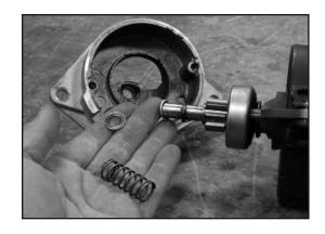
Note the retainer and cup washer on the end of the armature shaft. Leave the retainer C clip and cup washer on the shaft unless you are going to replace the starter drive. If there are any additional shim washers remove them and set aside for later.
