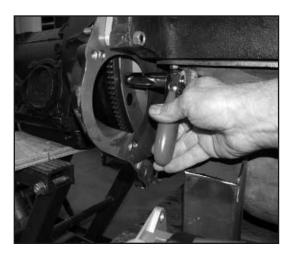
Tighten bellhousing nuts to 35 ft lbs and start a nut on the torque converter stud. Run nut down but do not tighten. Rotate crank and install the next converter nut, repeat until you have all 4 started, then torque to 35 ft lbs. Install starter to complete the job.
