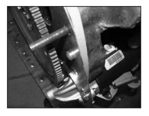
NOTE: at this time you might choose to do a visual check of the starter engagement. Position the starter up to the engine using the block plate to establish it's position. Do not allow the starter to hang on the block plate and bend it, insert a couple of bolts and note relationship of starter drive teeth and ring gear. Prior to installing the transmission, remove the torque converter retainer, if so equipped. Also remove the 3 nuts temporarily securing the block plate to the adapter.
