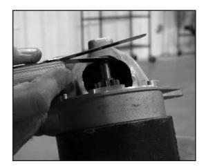
Stand starter up onto the base plate. Check the clearance between the cup washer and the starter snout. If the gap exceeds the thickness of one of the shim washers, remove starter snout bolts and install one of the previously removed shim washers. Reassemble and check end play.
