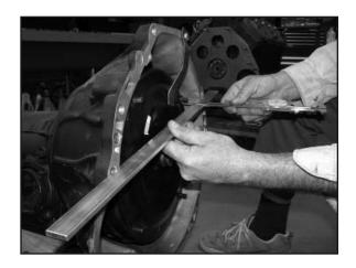
If you are using a complete transmission assembly purchased from Speedway or another reputable company, there is normally a support strap installed to keep the torque converter properly engaged during shipping. Leave this strap in place to take the following dimensions.
