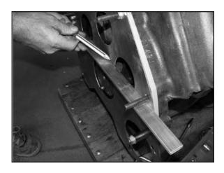
Using a straight edge (a length of 1/4"x1" flat stock works well) make sure that the block plate is absolutely flat. Depth measurements will be taken off of this surface and it is critical that the plate is not bent or distorted.
