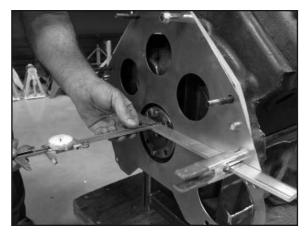
Using your straight edge and a machinist rule or caliper, take a depth check from the block plate to the crank hub. This dimension should be .150" +/- .020. (be sure to subtract the width of your straight edge from the indicated dimension) If this dimension is out of limits, check that the adapter is correctly seated, or if there is excessive end play of the crankshaft due to worn main bearings.
