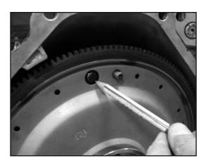
Check that the pilot hub of the torque converter fits properly in the center hub of the flywheel. If it is too tight, remove any rust or paint and Apply a small dab of grease to the center of the hub to make sure converter pilot does not bind. Also check that all 4 converter studs and the converter drain plug are aligned properly.
