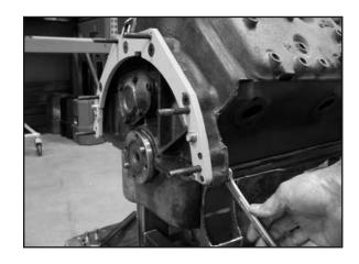
Secure the adapter plate to the engine with the supplied flat head screws. Note that one screw has the head turned down to clear the adjacent trans stud (@ approximately the 2 O'clock position. Also use 2 ea 3/8" nuts on the lower studs to secure to the block.
