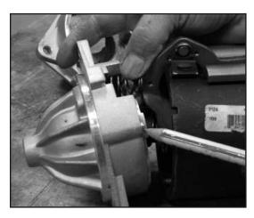
Apply a dab of grease to the end of the armature shaft and install the new snout over the shaft and starter drive, making certain that the return spring is inserted correctly. Align the dowel pin with the recess in the starter case and reinstall bolts.
