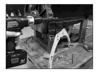
The two lower holes of the bellhousing mount flange on the block must be drilled out to 13/32" to accommodate the forward study of the transmission adapter plate.
