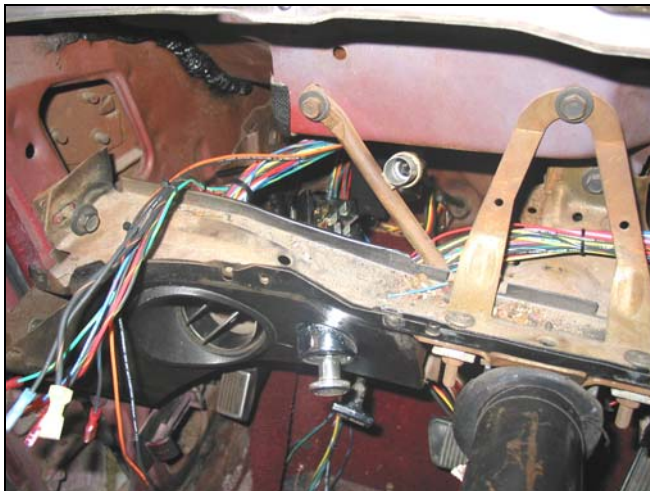
Figure 6-9 Interior Section Routing
