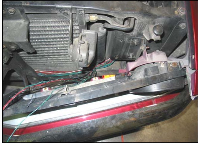
Figure 6-7B Headlight Section Routing
