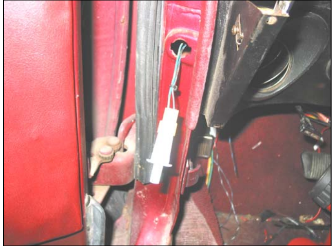
Figure 7-13 Door Jamb Switch
