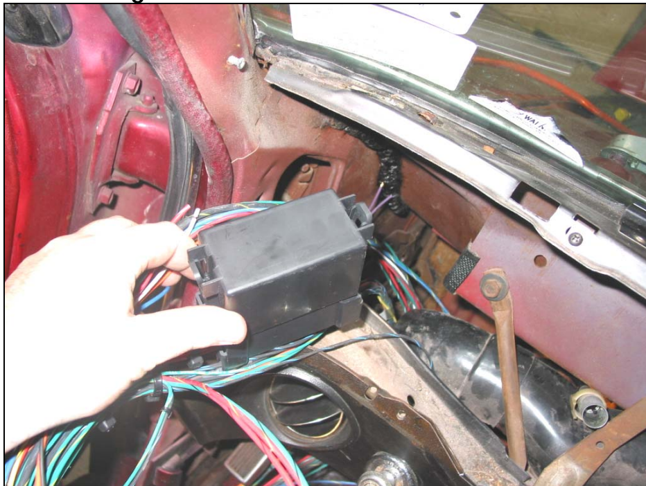
Figure 6-3 Routing Fuse Block through Instrument Cluster Opening
