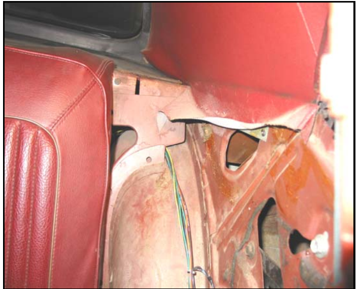
Figure 6-8D Tail Section Routing
