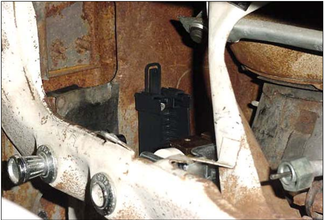
Figure 2 Fuse Block Base Mounting
