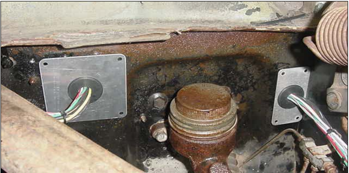
Figure 4 Pass Through Plates and Grommets
