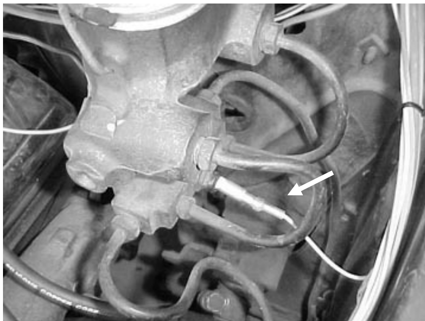
Figure 8.16 Brake Pressure Warning Switch Connection
