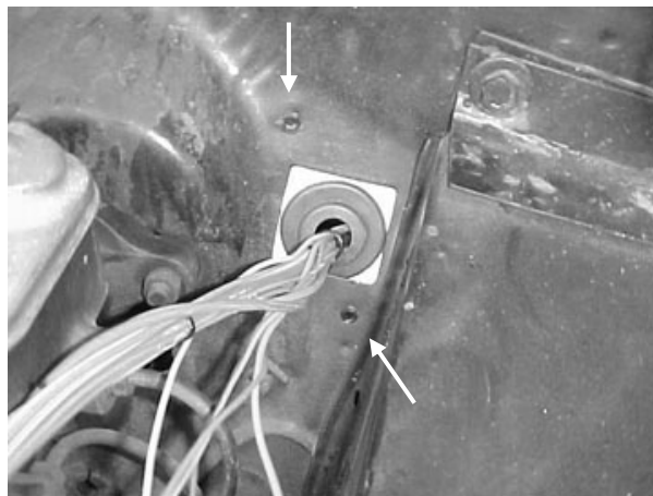
Figure 8.2 Screws Securing Adapter Bracket
