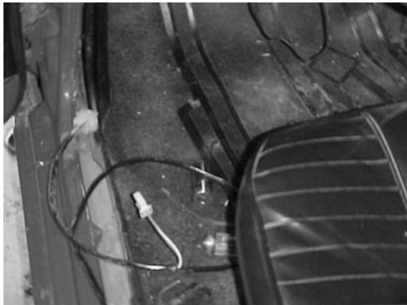
Figure 8.6 Driver Kick Panel and Jamb Routing
