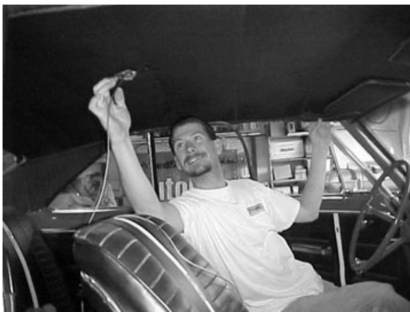
Figure 8.4 Routing Dome Light Wires
