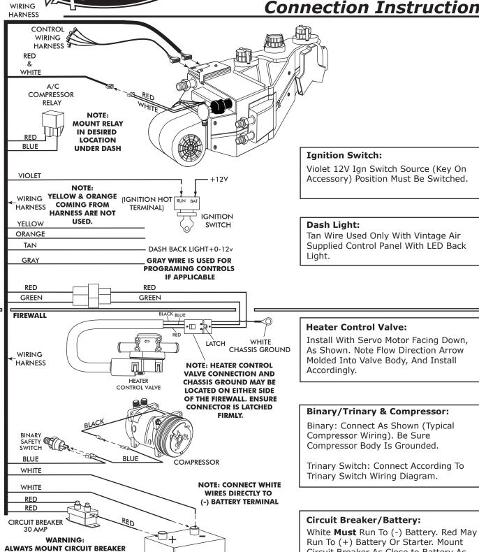
Run To (+) Battery Or Starter. Mount Circuit Breaker As Close to Battery As Possible.
