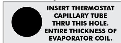
INSERT THERMOSTAT CAPILLARY TUBE THRU THIS HOLE. ENTIRE THICKNESS OF EVAPORATOR COIL.
