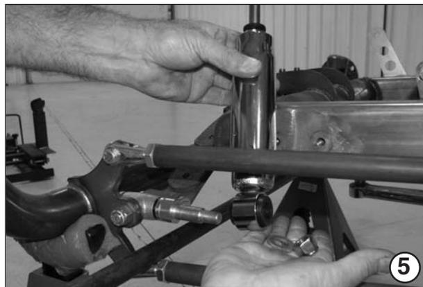
6) Position upper shock / heading mount bracket on frame rail. Determine which shock mount hole best suits your particular application.
