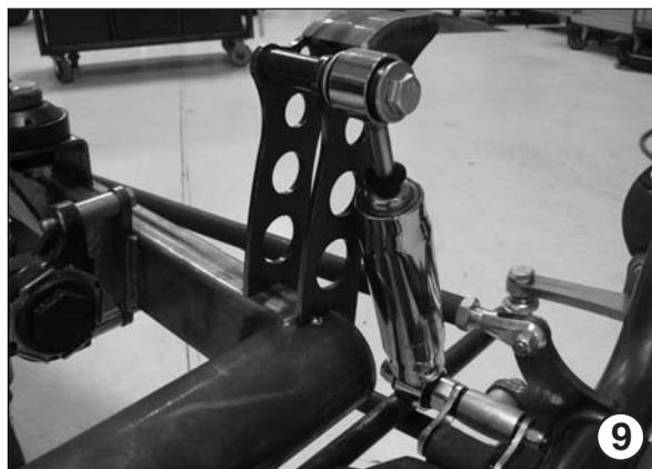
9) Check shock travel and suspension movement, look closely for interference with any moving suspension or steering components. If all is satisfactory, finish weld brackets to frame and tighten all fasteners to recommended torque.
