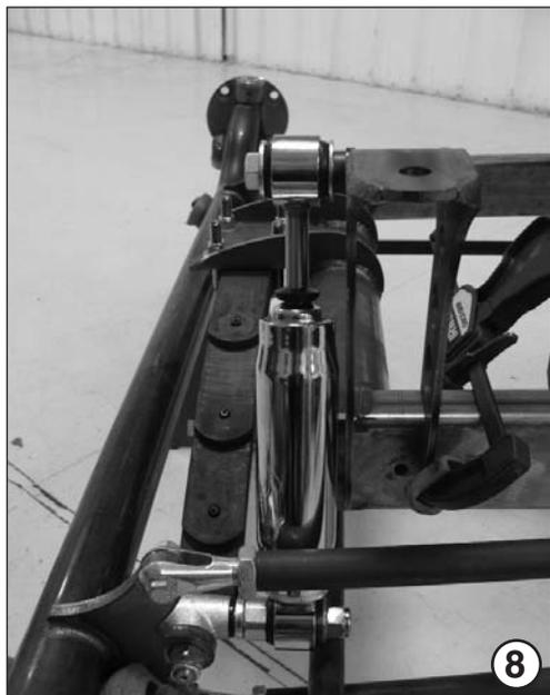
8) Make sure that the upper shock mount bracket sits squarely on the frame rail. Double check alignment of the shock. Clamp bracket in place and tack weld.
