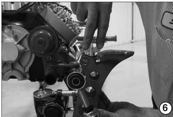
7) Secure the threaded bushing into the shock mount in the desired location using the button head cap screw in the AFT side of the shock mount. Install the upper shock bolt, washers, and spacer onto the front side of the shock mount bracket. Hand tight only.
