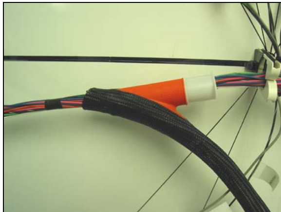
The “spreader” of the tool is then inserted into the PowerBraid. With the tool inserted, pull the tool down the length of the PowerBraid. This will insert the harness into the braid as it is pulled.
