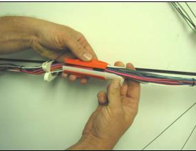
The wire is inserted into the tool. The tool is then closed around the wire
