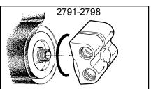
in the engine adapter ports. Seal the threads with Teflon® tape or appropriate sealer on pipe thread style fittings. Note: if installing AN or SAE fittings, **DO NOT** use any type of sealer on threads. MAXIMUM TORQUE on the fittings is 28 ft. lbs. (38Nm). DO NOT OVERTIGHTEN! Re-install the adapter. Tighten by hand 1/4 to 1/2 turn past O-Ring contact with sealing surface, about 20 ft. lbs. (28Nm).
