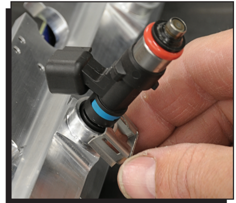
Figure 6 Installing the Injectors.
