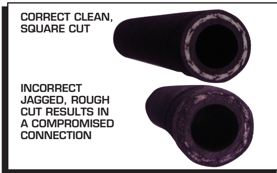
Figure 12 Severing the Hose Properly.
