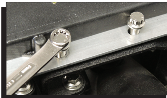
Figure 8 Tighten the Fuel Rail Bolts.
