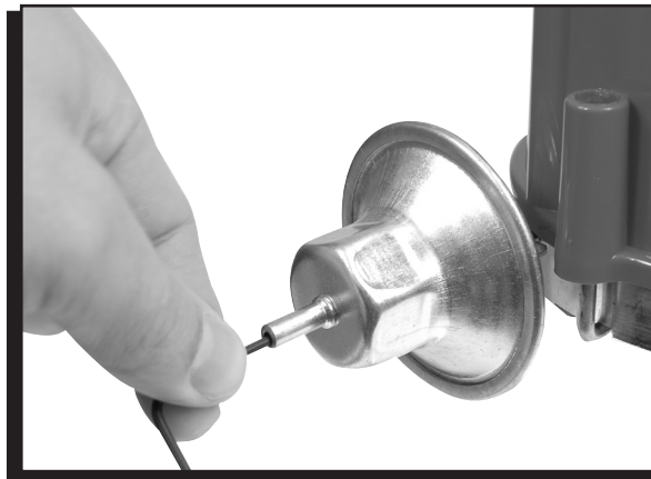
Figure 3 Adjusting the Vacuum Advance.
