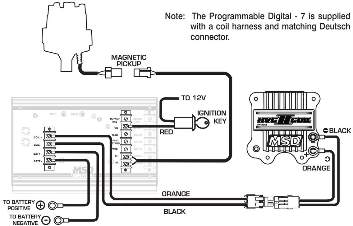
**WARNING:** Very high voltages are present at the coil when the engine is running. Never connect any test equipment or touch the coil while the engine is cranking or running.
