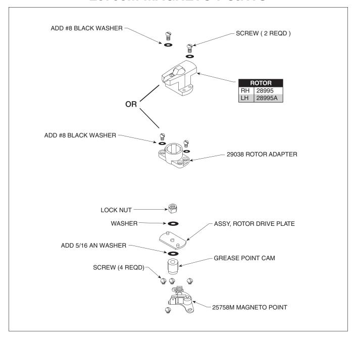
Hold 4 pin driver on bottom of magneto head and remove lock nut, as seen on diagram. Now remove lock washer, rotor drive plate and grease point cam. Next, install 5/16 AN washer, followed by drive plate, lock washer and lock nut. Install #8 black washers on rotor screws. Be sure to adjust point to .016". Double check this gap after about 30 minutes of running time.
