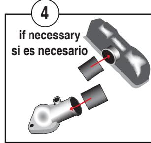
4. Measure your radiator outlets and water pump or thermostat housing. If your outlets are 1-1/4" or 1-1/2", install the provided adapter onto the outlet (not into the insert). If they are 1-3/4" no adapter is necessary.
