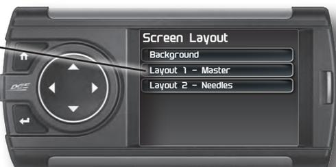
**STEP 4** - Use the Up/Down buttons to scroll through the available screen layouts. Press Enter to select an option.
