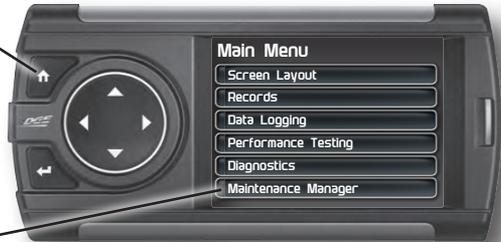
**STEP 2** - Use the Up/Down arrow buttons to scroll down to the Maintenance Manager option.
