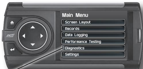
**STEP 2** - Use the Up/Down arrow buttons to scroll down to the Diagnostics option.
