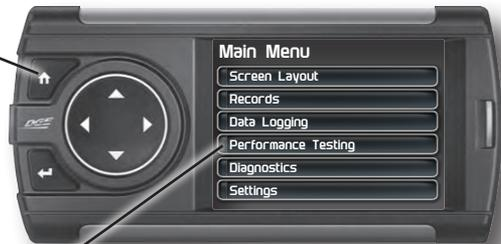
**STEP 2** - Use the Up/Down arrow buttons to scroll down to the Performance Testing option.
