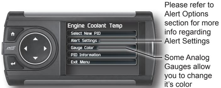
**STEP 6** - Return to the main gauge screen. The new PID will be displayed along with any customized options you may have changed.
