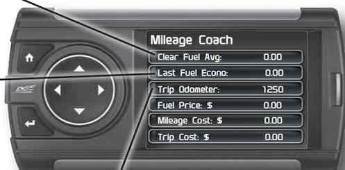
The Trip Odometer is used to calculate the Trip Cost and Fuel Average.
