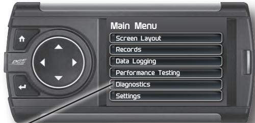
**STEP 2** - Use the Up/Down arrow buttons to scroll down to the Diagnostics option.
