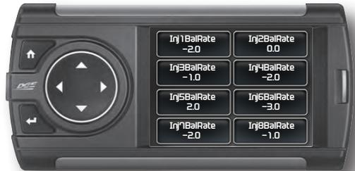
If you suspect a faulty injector, we recommend consulting a professional diesel mechanic who can verify the issue and also perform a cylinder power balance test to further diagnose.
