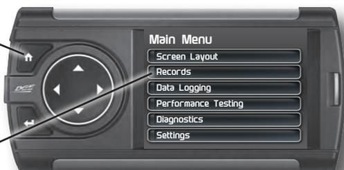
**STEP 2** - Use the Up/Down arrow buttons to scroll down to the Records option. Press Enter.
