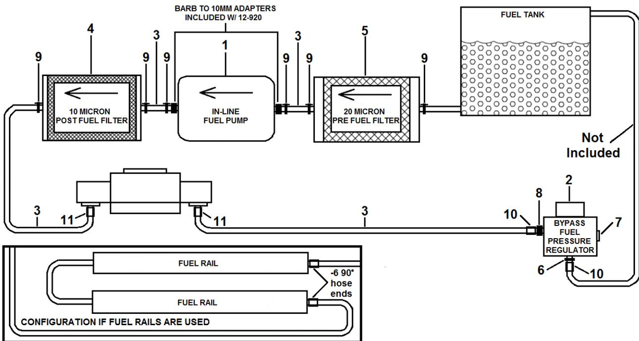
Figure 3 – KIT 526-4 (refer to 4.2 PARTS IDENTIFICATION)
