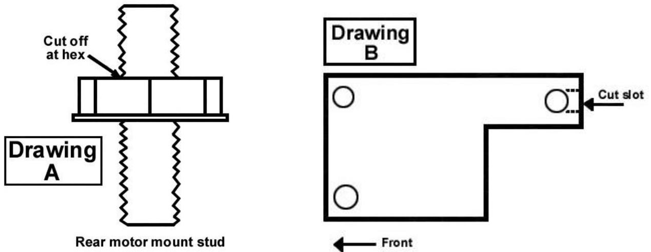
15. After the mount has been modified, insert it back into the engine bay. Do not mount at this time.
