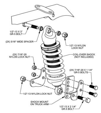
is design to use 4" stroke shocks with a compressed length of 10"-11" and an extended length of 14"-15". Shock ends should be ½" bearings with a mounting width of 1". For recommended part numbers please visit our website or contact one of our tech experts.
