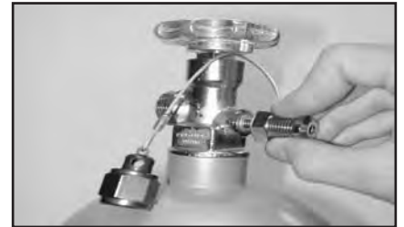
Hand-tighten the PRD into place as shown above paying special attention to making sure the Burst Disc remains in place. Once hand-tight, torque to 17 ft. lbs. using a properly calibrated torque wrench.
