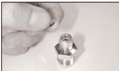
Shown above is the new burst disc being installed on the Racer Safety Blow Off Adapter. Be sure when installing the burst disc that you do not collapse the sides of the disc or damage the disc in any way.
