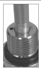
Apply a small amount of red Loctite to siphon tube threads and install on valve.
