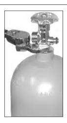
Install the bottle valve and siphon tube assembly on bottle. Torque valve to 90ft/lbs.
