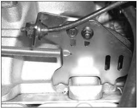
Figure 2 - Throttle Cable Bracket
