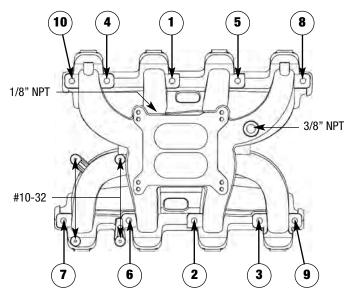
Figure 1 - Intake Manifold Tightening Sequence
