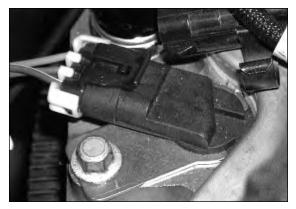
Figure 6 - Camshaft Position Sensor
