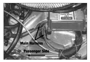
Figure 4 - Timing Control Module Mounting
