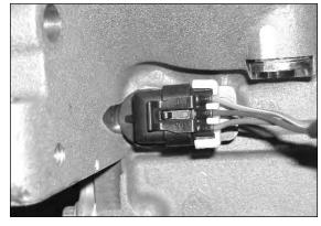
Figure 5 - Crankshaft Position Sensor
