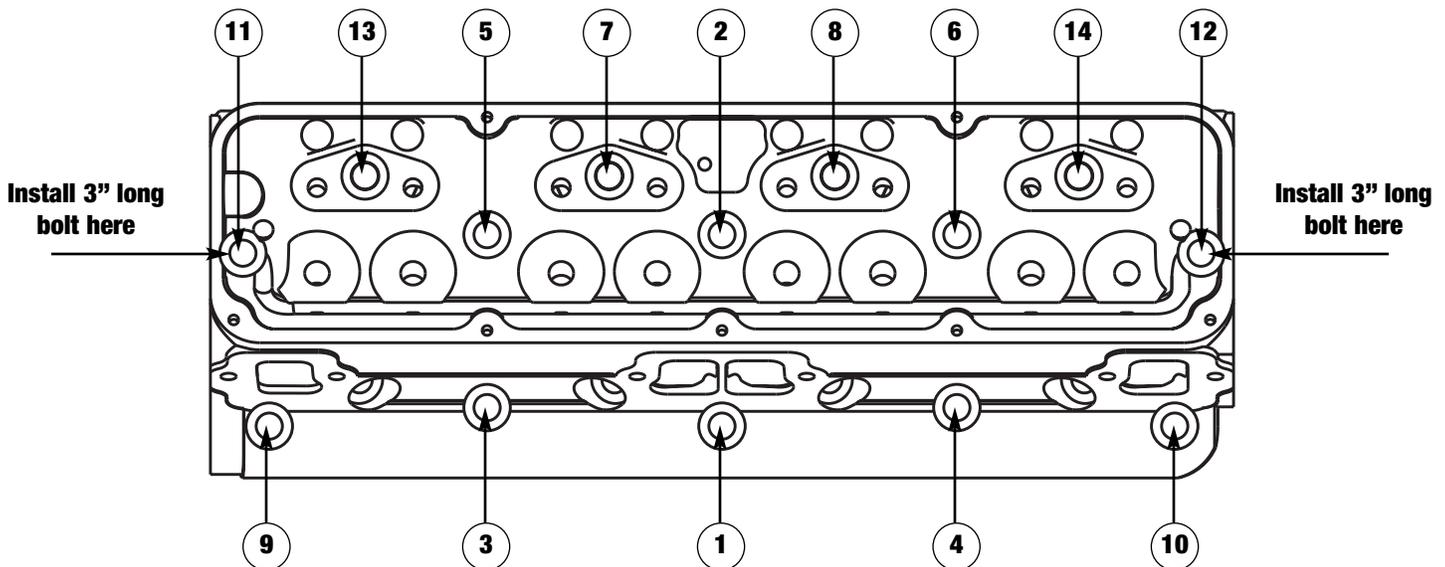
**Figure 1 - AMC Cylinder Head Bolt Tightening Sequence**
