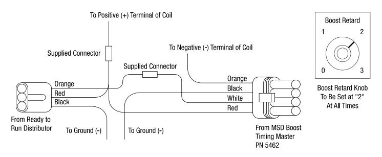
**NOTE:** The included MSD Boost Timing Master is pre-set for the E-Force RPM Supercharged crate engine at 2° of timing retard per pound of boost. The knob should not be adjusted to any other setting except "2".
