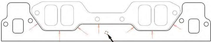
**NOTE #1:** Both intake manifolds and valley plates have been designed to fit multiple cylinder head and deck height combinations when final machining is performed to desired dimensions. Lower flange surfaces and/or the corresponding surfaces of the valley plate may require additional machining for proper manifold to valley plate clearance. This work should only be performed by a qualified engine builder or machinist.
