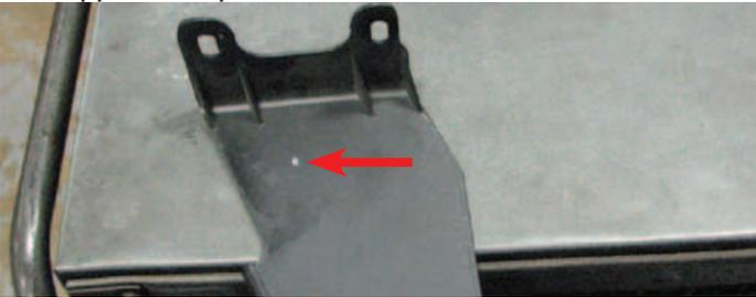
131. Use a 10mm socket and the four stock bolts to reinstall the upper radiator shroud then attach the relay off the supplied water pump wire harness to the upper radiator shroud using the supplied body pin. Open and close the hood to verify the relay clears the hood strut.
