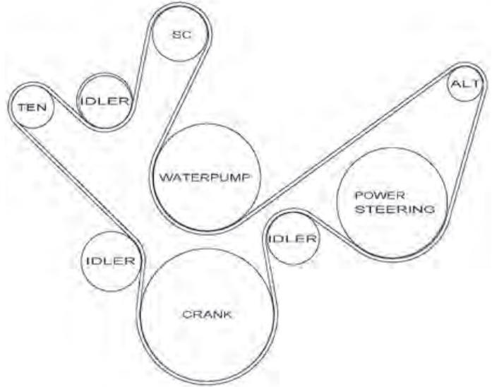
187. Use a breaker bar and a 16mm socket to push the tensioner enough to get the belt on, then double check the routing.
