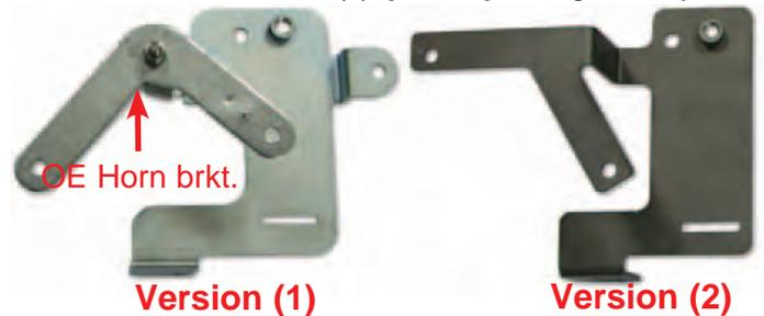
128. **NOTE: This step only applies to customers who received version (1) of the water pump brackets.** Install the supplied stand-off and lock nut onto the OE horn bracket. Proceed by mounting that assembly, with the supplied M6 x 10mm bolt, to the water pump bracket as shown below.
