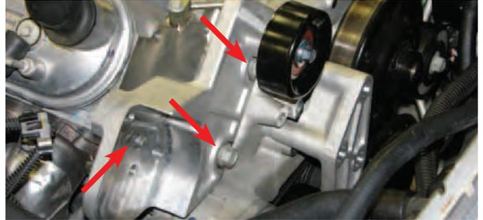
110. Use an 8mm allen tool to install the 45mm bolt supplied in Bag #1 that retains the tensioner bracket to the cylinder head and torque it to 37 ft-lbs.
