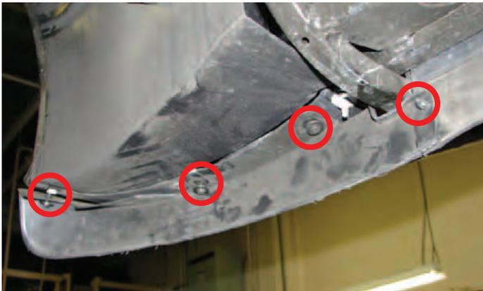
11. Remove the five 7mm and two 10mm nuts retaining the fascia from below.
