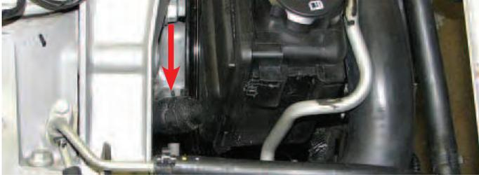
115. Slide the old bracket off the reservoir then install the supplied bracket using a 15mm socket and the stock bolts. Slide the power steering reservoir onto the new bracket and reattach the lower reservoir to pump hose.
