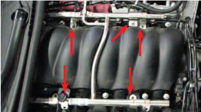
30. Lift the injectors out of the manifold and work the rails forward until they can be set aside.
