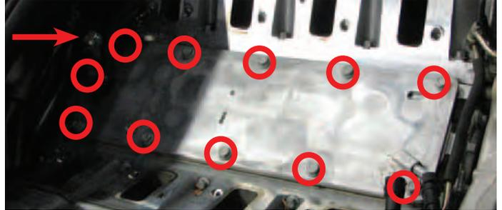
43. Clear engine valley of all debris then use a 13mm socket to remove the 11 bolts retaining the valley plate and remove it.
