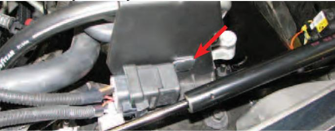
132. Route the intercooler water pump wire harness extending from the relay down to the intercooler water pump and plug in the connector.
