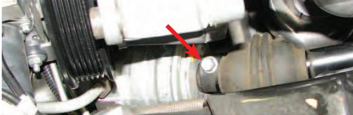
59. Use a 6mm Allen tool to hold the tie rod ball stud stationary while using an 18mm wrench to loosen the nut.
