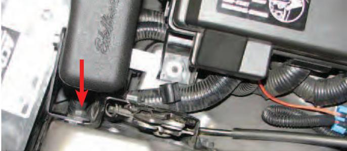
146. Install intercooler reservoir by working molded hose down along the passenger side of the radiator to the water pump inlet and secure the hose on the pump fitting with a hose clamp supplied in Bag #2.
