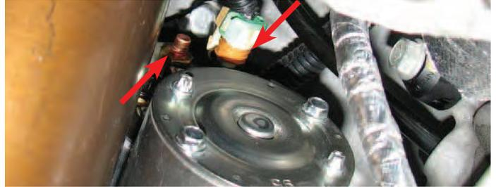
81. Use a 13mm socket to remove the nuts retaining power wires to the starter.
