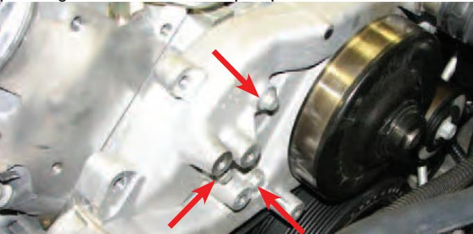
108. Use a 2" long 6mm Allen socket and the three 90mm bolts supplied in Bag #1 to install the lower idler bracket on the water pump, then torque them to 18 ft-lbs.
