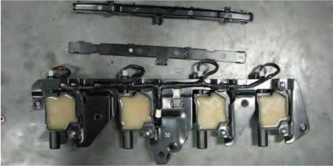
176. Tuck the fuel injector wiring harness and the EVAP Solenoid to Firewall Fitting Hose between the valve cover and manifold then use a 10mm socket and the ten stock bolts to install both coil brackets on to the valve covers. Pull the wiring harness on the passenger side forward to provide enough slack to attach the TPS harness connector.
