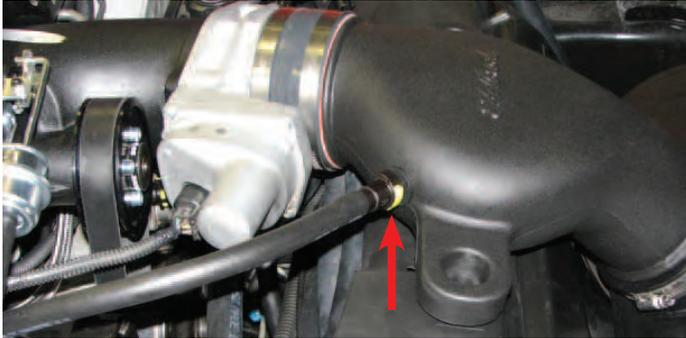
201. Rotate the worm clamps so that the gears are on the driver side then secure the air inlet tube by tightening the worm clamps on the air filter and the silicone hose.
