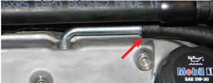
171. Install the supplied driver side PCV hose to the 90° fitting below the air inlet on the supercharger.
