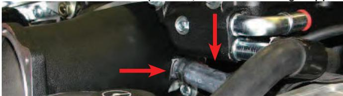
159. Use a 10mm universal socket with an extension bar to install the eight intake manifold bolts following the torque sequence below. Torque the bolts to 4 ft-lbs in the first pass, then to 7.5 ft-lbs in the second.
