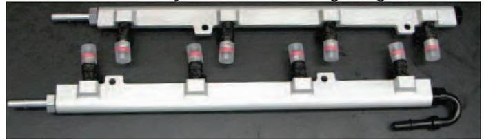
163. Apply O-ring lube to the sealing ring of the four supplied fuel rail fittings. Use a 3/4" wrench to install the two straight hose fittings on the radiator side of each fuel rail then install the plug in the firewall end of the passenger side fuel rail and the U-shaped fitting on the firewall end of the driver side rail. Orient the fitting close to the injector, leaving room for the injector connector.
