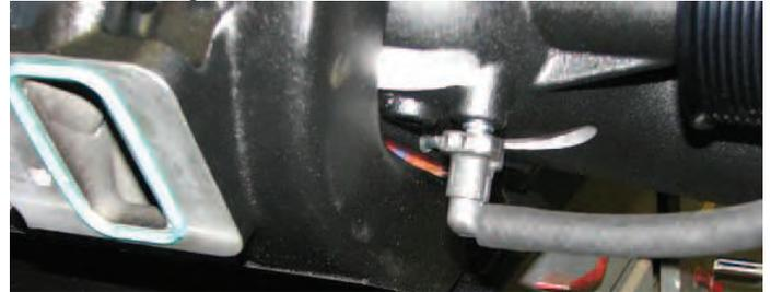
155. Remove the water passage block-off located at the rear of the driver side cylinder head. Grind a 1/4" of material off the inside corner of the block-off at a 45° angle, then reinstall it .
