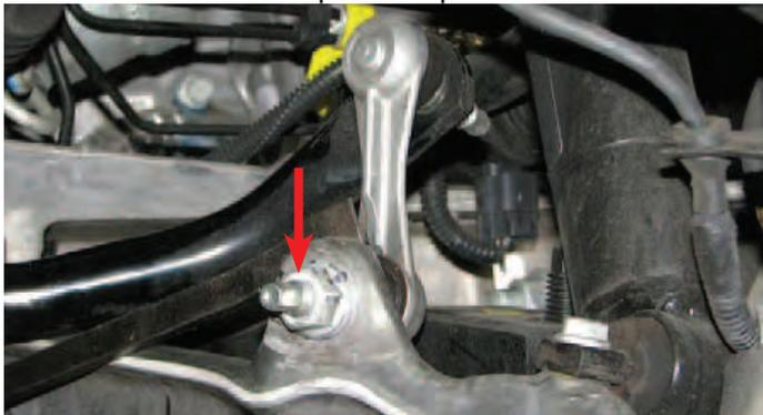
62. Use a 13mm socket to remove the four bolts retaining the stabilizer brackets.
