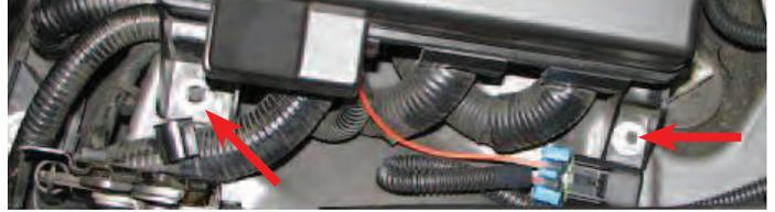
141. Use a 10mm socket and an extension bar to loosen the two nuts securing the fuse box.
