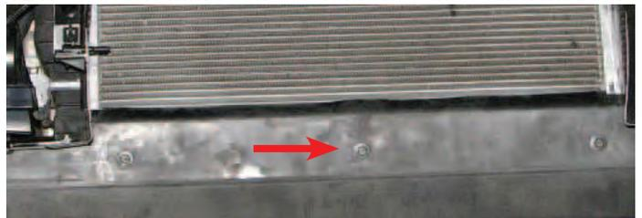
122. Use a 10mm socket to install the heat exchanger, using the 20mm bolts supplied in Bag #2 on the side, and the stock air dam bolt on the bottom.
