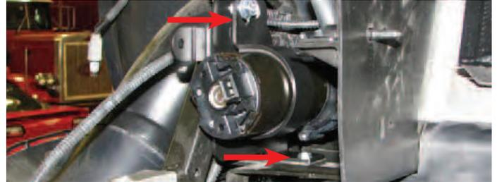
NOTE: There are two different water pump brackets: Version (1) requires the use of your OE horn bracket. Version (2) has an integrated horn bracket. You should have received one of the two brackets; If your supercharger kit includes bracket version (2), you may disregard Step 128.
