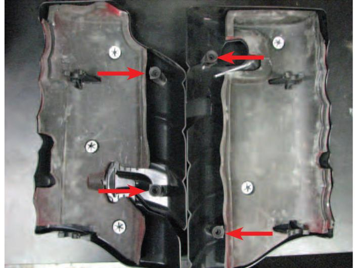
180. Install the stock grommets into the coil cover brackets supplied in Bag #6.
