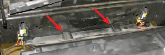
53. Disconnect the radiator fan electrical connector then use a 10mm socket to remove the two bolts retaining the fan assembly. Pull the hoses from the six clips holding them to the assembly and remove the fan from below.
