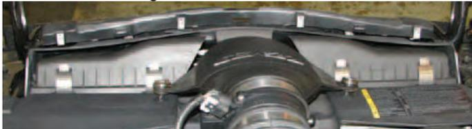
24. Disconnect the ignition coil harness and O2 sensor connectors then disconnect the spark plug wires from the ignition coils.
