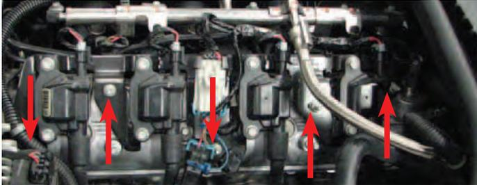
26. Use a fuel line removal tool to disconnect the fuel line from the rails using a shop rag to absorb excess fuel.
