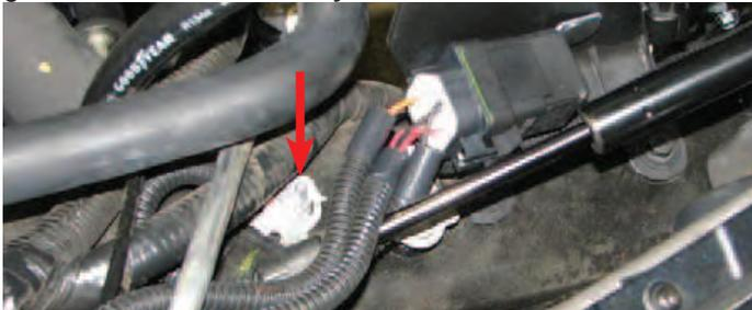
151. Reinstall the fender well fuse box bolt.
