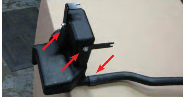
144. Use a 10mm socket to install the brackets supplied in Bag #2 on the reservoir. The image above shows the installed orientation.
