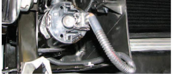
133. Plug the male connector on the T-segment of the harness into the EVAP solenoid then plug the factory EVAP connector into the female connector on the T-segment.
