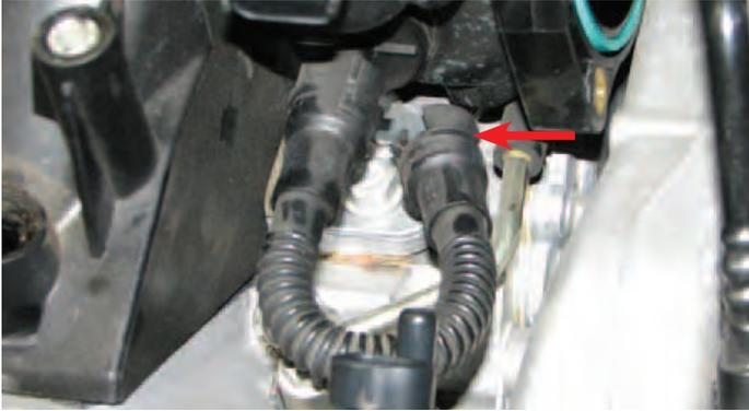
37. Remove the intake manifold and disconnect the small vacuum hose at the rear of the manifold next to the larger brake booster hose, if it is present. Leave this hose hanging from the firewall as it will be reconnected later.
