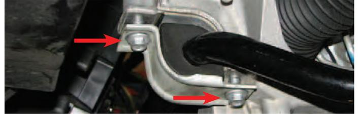
63. Use a 13mm socket to remove the two nuts retaining the brake pressure modulator valve.
