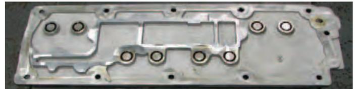
45. Apply anti-seize to the tapered surface beneath the heads of the countersunk bolts supplied in Bag #3 and install the valley plate with the stock gasket. Tighten the bolts from the center out with a 5mm allen tool then torque them to 18 ft-lbs in the same sequence.
