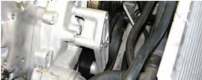
109. Use a 15mm socket and the two stock bolts to mount the new tensioner bracket onto the water pump then torque them to 37 ft-lbs.
