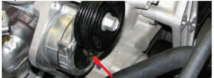
113. Use a 12mm socket and a 20mm bolt supplied in Bag #1 to mount the EVAP purge solenoid on the back of the new tensioner bracket.
