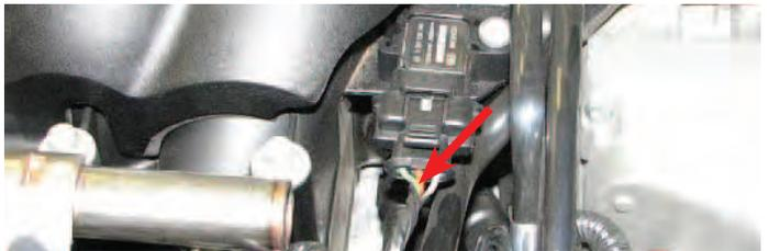
34. Disconnect the vacuum hose from the brake booster fitting; it will be removed with the manifold.
