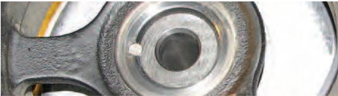
89. Install the supplied GM crank bolt into the crank and torque it to 37 ft-lbs, then rotate it an additional 140°.
