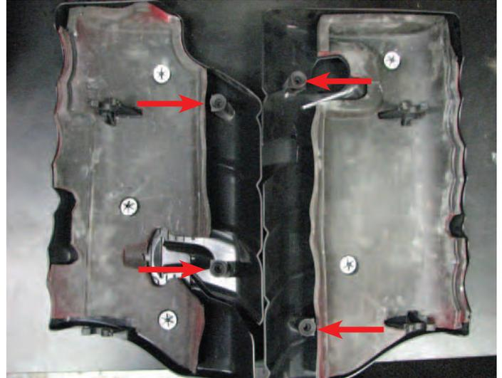
177. Install the stock grommets into the coil cover brackets supplied in Bag #6.
