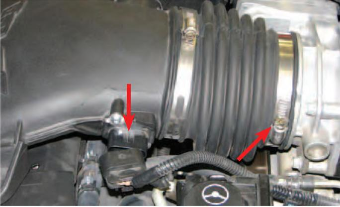
16. Use a flat head screwdriver to loosen the Throttle Body to inlet tube worm clamp.
