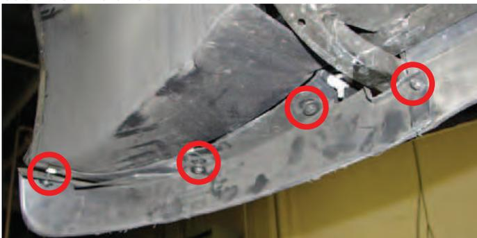
11. Remove the five 7mm and two 10mm nuts retaining the fascia from below.
