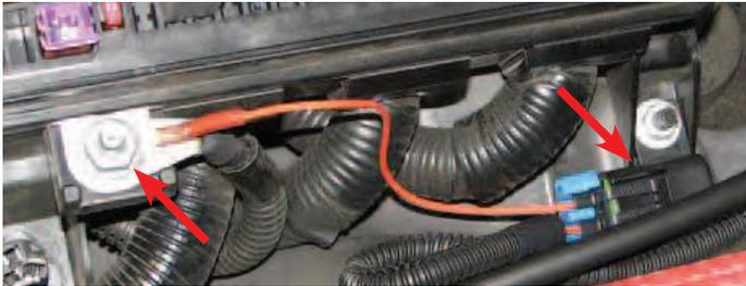
147. Use a 13mm socket to attach the harness power wire to the main positive terminal.
