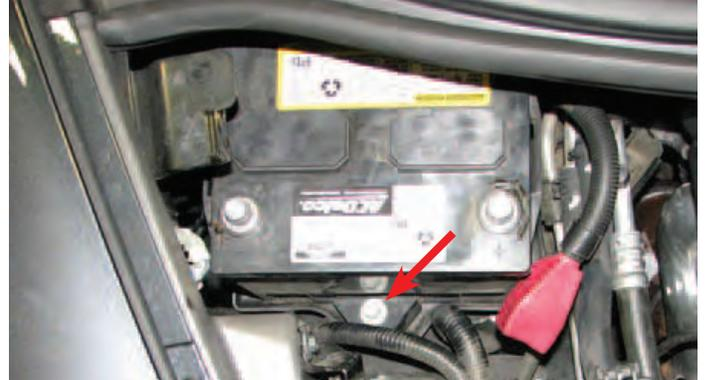
4. Remove the battery and set it to one side.
