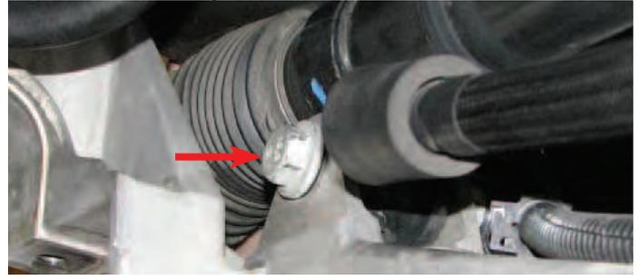
74. Loosen the rear engine cradle nuts with a 21mm deep socket and lower them until there is a gap of 10mm from the cradle to the top of the nut.
