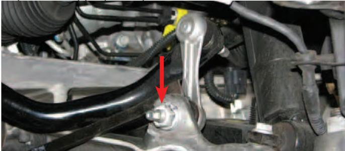
62. Use a 13mm socket to remove the four bolts retaining the stabilizer brackets.
