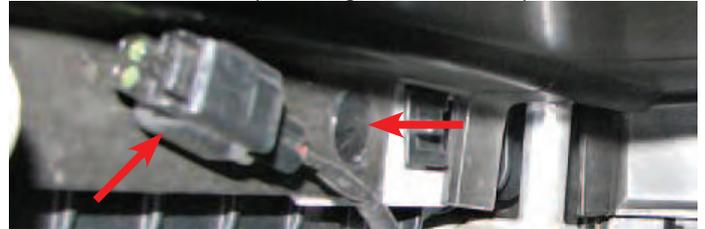
51. Disconnect the ambient air temperature sensor and remove the sensor clipped to passenger side of shroud.
