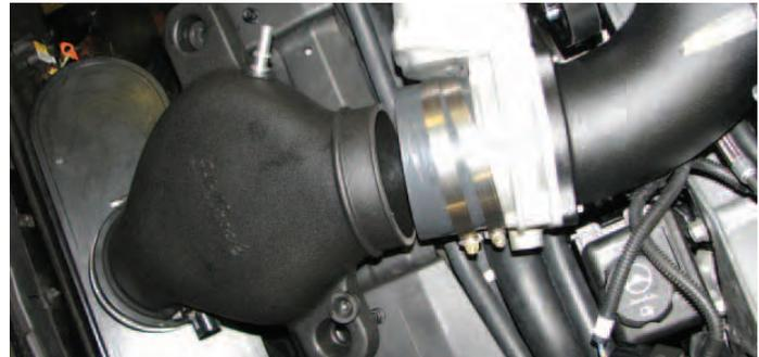
196. Slide the nose of the air inlet tube into the air filter then hold the grommets in place with a socket as you tilt the air inlet tube down into the silicone tube and onto the locator pins.
