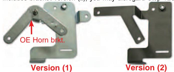
126. NOTE: This step only applies to customers who received version (1) of the water pump brackets. Install the supplied stand-off and lock nut onto the OE horn bracket. Proceed by mounting that assembly, with the supplied M6 x 10mm bolt, to the water pump bracket as shown below.
