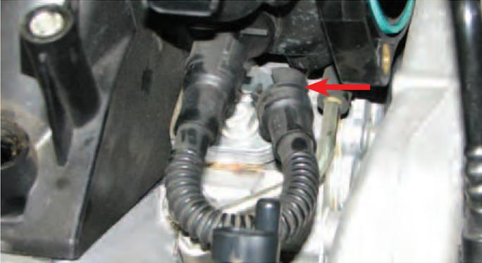
37. Remove the intake manifold and disconnect the small vacuum hose at the rear of the manifold next to the larger brake booster hose. Leave this hose connected to the firewall as it will be reused later.
