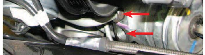
65. Use a 10mm socket to remove the bolts retaining the power steering line brackets or fluid cooler, if equipped.
