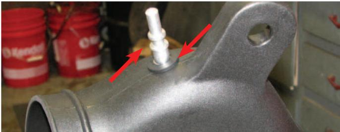
190. Install the hose barb supplied in Bag #5 into the new air inlet tube.
