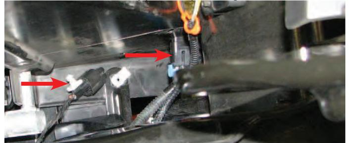
52. Reach up from below the car to remove the two remaining body pins retaining the front radiator shroud then remove the shroud by pulling it down and out.
