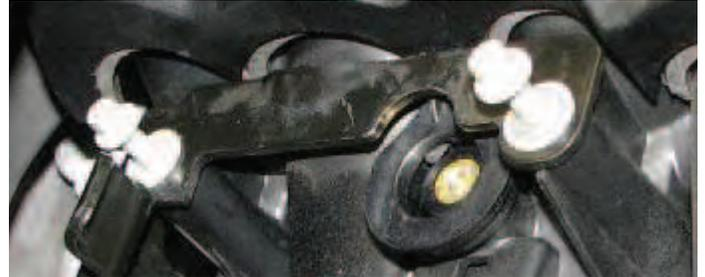
31. Use a 10mm socket to remove the seven remaining manifold bolts (out of ten).
