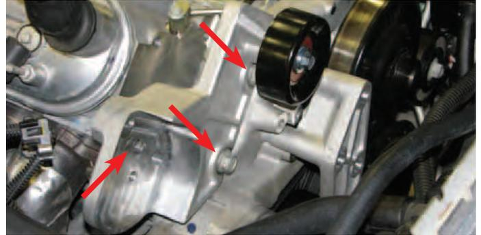
111. Apply blue loctite to the threads of a 20mm bolt supplied in Bag #1, then use a 12mm socket and the supplied washer to mount the pulley on the tensioner bracket and torque it to 18 ft-lbs.
