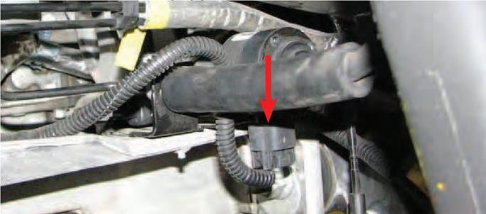
69. Use a 10mm socket to remove the driver side brake line bracket bolt.
