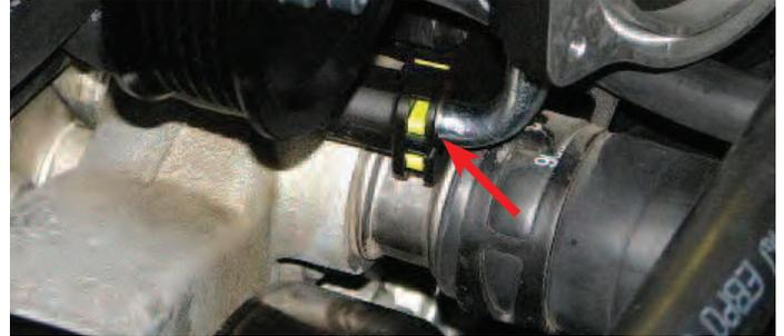
169. Install the supplied fuel line from the firewall fitting to the U-shaped fitting on the driver side fuel rail.
