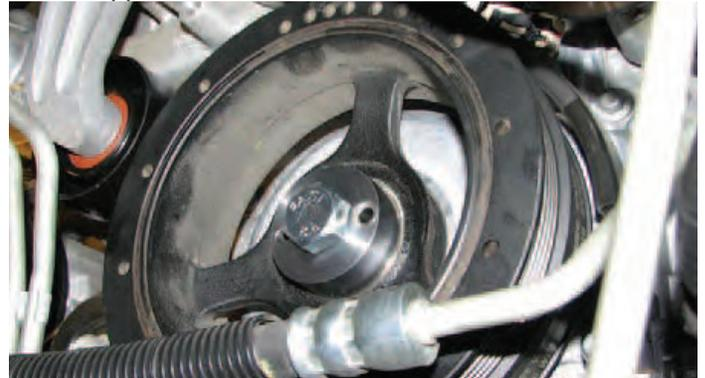
86. Use a 24 mm socket to install the supplied bolt and reamer guide to the end of the crank.
