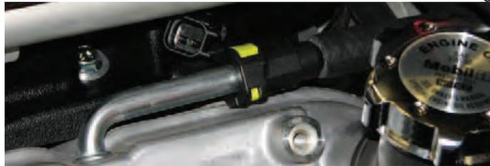
168. Install the supplied driver side PCV hose to the 90° fitting below the air inlet on the supercharger.
