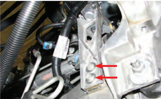
72. Use an 18mm socket to remove the two steering rack nuts and bolts.
