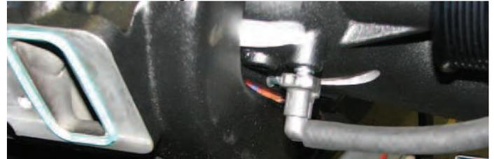
153. Clear engine valley of any hoses, wires, tools, etc. Lay the intercooler-to-reservoir tank hose in the engine bay, routed along the firewall behind the oil pressure sensor, and connect it to the intercooler reservoir inlet, securing the fitting with a hose clamp supplied in Bag #2.
