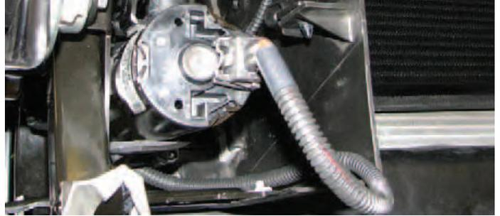
131. Plug the male connector on the T-segment of the harness into the EVAP solenoid then plug the factory EVAP connector into the female connector on the T-segment.
