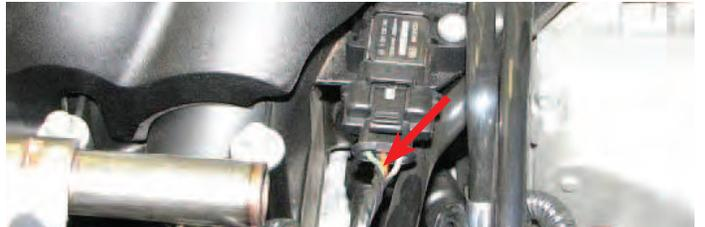
34. Disconnect the vacuum hose from the brake booster fitting; it will be removed with the manifold.
