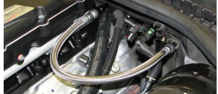
170. Connect fuel injector electrical connectors.
