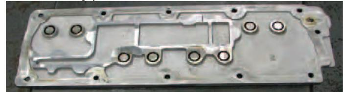
45. Apply anti-seize to the tapered surface beneath the heads of the countersunk bolts supplied in Bag #3 and install the valley plate with the stock perimeter gasket. Tighten the bolts from the center out with a 5mm allen tool then torque them to 18 ft-lbs in the same sequence.
