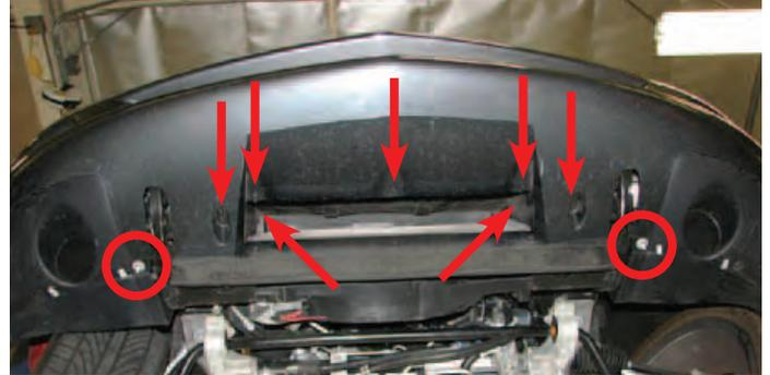
12. Remove four body pins (two on each side) by reaching up through the bottom of the fascia.
