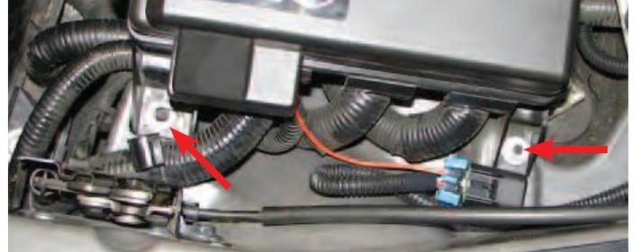
140. Use a 7mm socket to remove the fuse box bolt located in the passenger side fender well.
