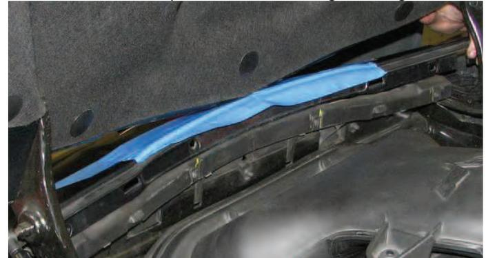
14. The sides of the fascia can be pulled away from the clips holding it in place, then down off the studs. The center section must be pulled up and over the nose section, and the whole assembly pulled straight off and set aside.
