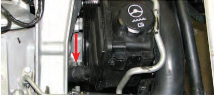
115. Slide the old bracket off the reservoir then install the supplied bracket using a 15mm socket and the stock bolts. Slide the power steering reservoir onto the new bracket and reattach the lower reservoir to pump hose.
