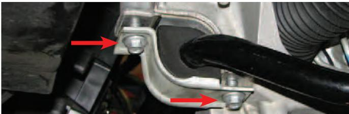
63. Use a 10mm socket to remove the two nuts retaining the brake pressure modulator valve.
