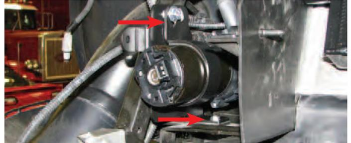
NOTE: There are two different water pump brackets: Version (1) requires the use of your OE horn bracket. Version (2) has an integrated horn bracket. You should have received one of the two brackets; If your supercharger kit includes bracket version (2), you may disregard Step 126.
