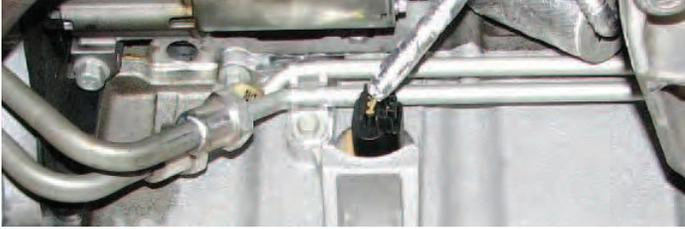
78. Use a 10mm socket to remove the starter support bracket bolt.
