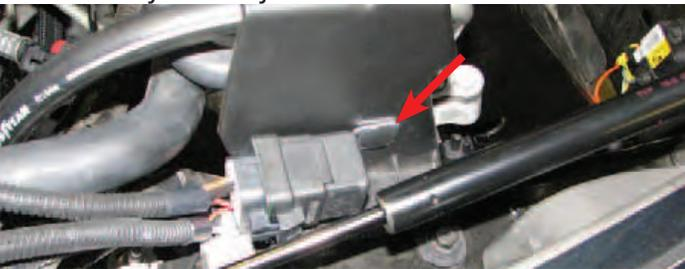
130. Route the intercooler water pump wire harness extending from the relay down to the intercooler water pump and plug in the connector.
