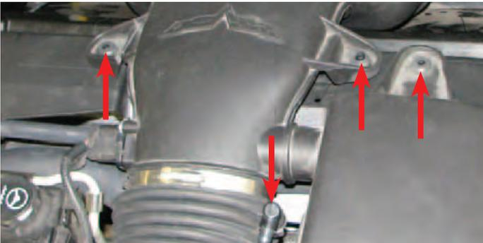
18. Lift the airbox and resonator tube off the locator pins and remove it and the air inlet tube as an assembly.
