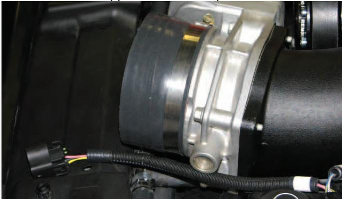
189. Install the grommet supplied in Bag #5 into the new air inlet tube.
