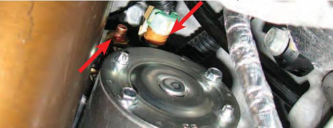
81. Use a 13mm socket to remove the nut retaining the power wire to the starter.
