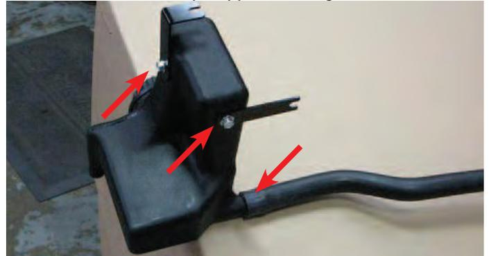
142. Use a 10mm socket to install the brackets supplied in Bag #2 on the reservoir. The image above shows the installed orientation.
