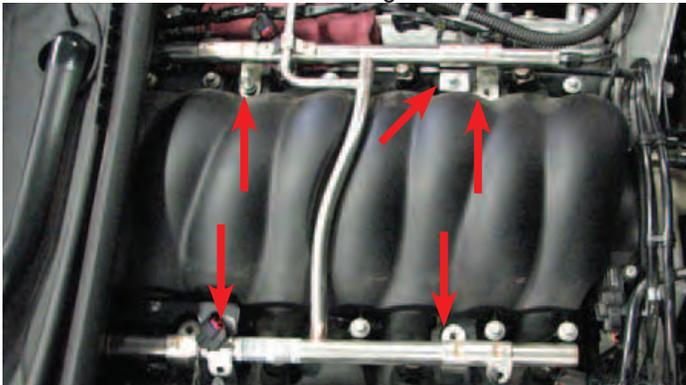
29. Lift the injectors out of the manifold and work the rails forward until they can be set aside.
