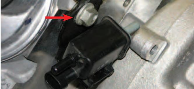
49. Use a 10mm socket to remove the four bolts (two on each side) retaining upper radiator shroud and remove it.
