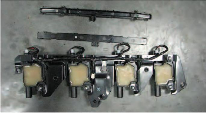
173. Tuck the fuel injector wiring harness and the EVAP Solenoid to Firewall Fitting Hose under driver side coil bracket then use a 10mm socket and the ten stock bolts to install both coil brackets on to the valve covers.
