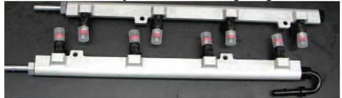
160. Apply O-ring lube to the sealing ring of the four supplied fuel rail fittings. Use a 3/4" wrench to install the two straight hose fittings on the radiator side of each fuel rail then install the plug in the firewall end of the passenger side fuel rail and the U-shaped fitting on the firewall end of the driver side rail. Orient the fitting close to the injector, leaving room for the injector connector.
