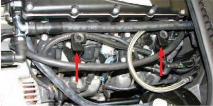
180. Tuck the wire harness tight against the fuel rails and route the driver side PCV hose on top of the driver side coil bracket and connect it to the valve cover fitting. 2008 vehicle owners will need to pull the quick connect fitting out of the supplied hose before attaching it to the valve cover fitting. Verify nothing will be pinched or damaged when the coil covers are installed.
