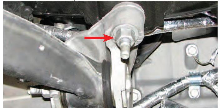
75. Insert a pry bar between the frame and front driver side cradle mount.
