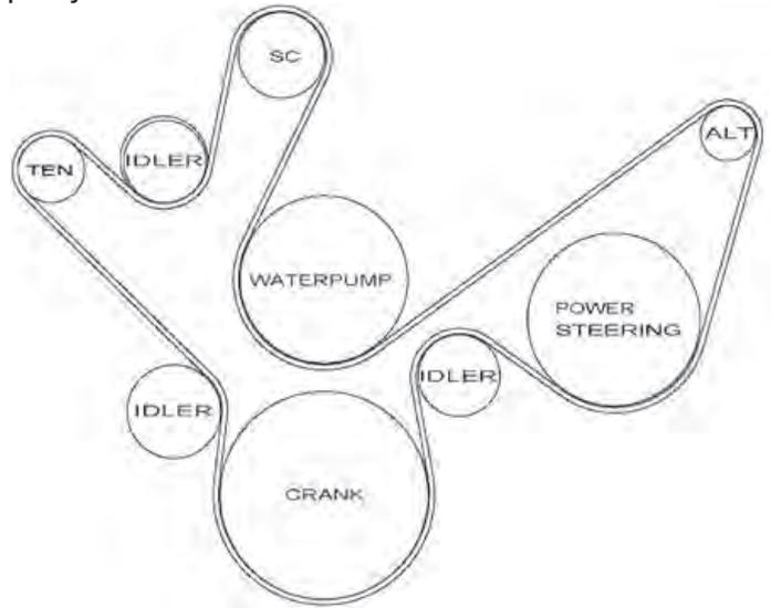
184. Use a breaker bar and a 16mm socket to push the tensioner enough to get the belt on, then double check the routing.
