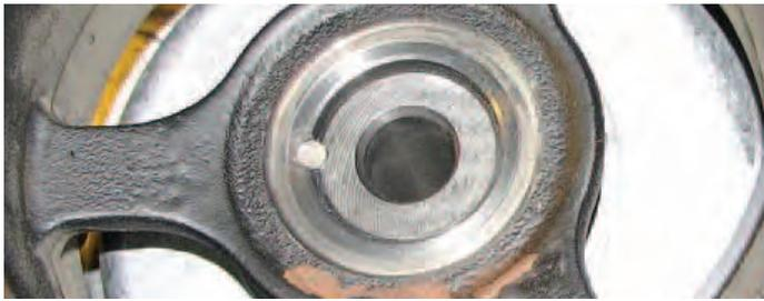
89. Install the supplied GM crank bolt into the crank and torque it to 37 ft-lbs, then rotate it an additional 140°.
