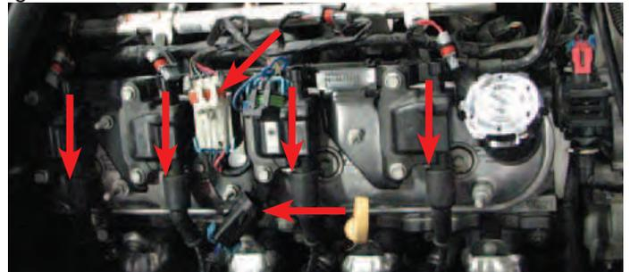
24. Use a 10mm socket to remove the five bolts retaining the coil bracket on each valve cover then remove both coil bracket assemblies.
