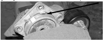
4. Use a grinding wheel or file to ensure that the area that was ground down is smooth and free of burrs.
