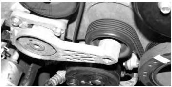
3. Place the tensioner in a cloth wrapped vice and use a grinding wheel or hacksaw to remove the stop.
