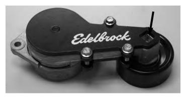
6. Use a 10mm socket to reinstall the tensioner.
