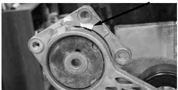
Part #15806 Rev. 10/10 - AJ/mc 5. Use a 10mm socket to install the three tensioner brace bolts, making sure to line up the square holes.
