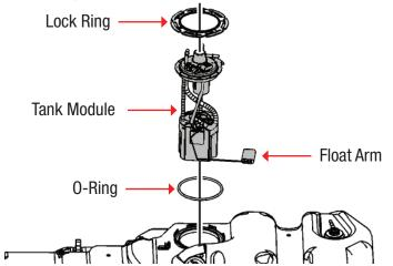
**NOTE:** Some lock rings were manufactured with "DO NOT REUSE" stamped into them. <u>These lock rings may be reused if they are not damaged or warped.</u>
