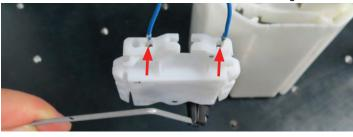
21. Install the sending unit onto the fuel pump module. Make sure the sending unit wires do not get pinched between the sending unit and the fuel pump module.
