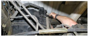
4. Place an adjustable jack under the fuel tank for support. Using a 15mm socket, remove both fuel tank strap bolts and straps.
