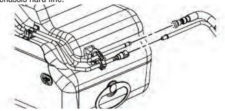
3. Disconnect the fuel tank EVAP line from the EVAP canister. Cap or tape up the fuel and EVAP lines to prevent possible system contamination.
