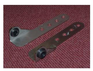
Prepare the angle brackets by inserting the supplied grommet through the large hole in the bracket. The muffler hanger should be greased lightly with white grease to ease the insertion through the grommet. Orient the hanger brackets so that the angle leg with grommet is to the outside of the vehicle. The bracket will be bolted into place through drilled holes with the supplied sheet metal screws after the clearance has been verified. (See the following steps)
