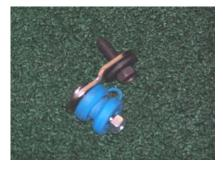
Note: Use a  $\frac{1}{4}$ " drill bit for the "body bolt" used to attach the offset tab to the frame or floor pan. This bolt extrudes the metal, forming a thread at is thicker than the metal thickness itself. Start the bolt, and then finish with a ratchet and socket or an impact
