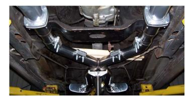
With all tubes and clamps in place, make sure that the interim tubes are leveled in the vehicle. Then begin the tightening process by fully tightening each of the four (4) bolts of each collector reducer. Then move back to the stainless steel band clamps and tighten them securely.
