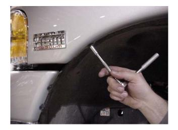
These screws need to be removed prior to removing both the LH and RH inner panels. This gives you lots of room to install your new headers. Is that a Hemi behind those panels?
