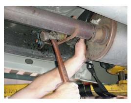
12. Loosen the nuts holding the "down tubes" to the cast manifolds .
