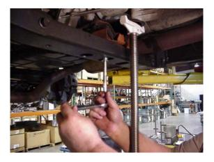
This shows the rear transmission housing support and removal of the transmission mounting bolt nuts.
