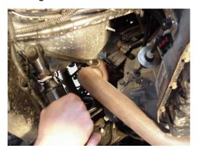
13. Before removing any cross member bolts, you must add a support to the transmission rear tail housing. Once supported, remove the 4 cross member bolts from the main frame brackets
