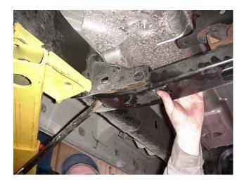
Pry the passenger side of the cross member down to aid in its removal.
