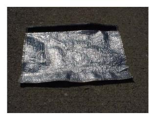
This thermal heat shield is to wrap around the fuel line and wiring harness going across from the frame to transmission just above the catalytic converter
