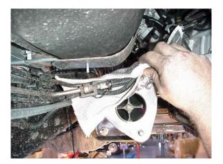
The reflective silver finish goes to the outside. Wrap the shielding material around the harness and fuel line and apply pressure to the Velcro strip.
