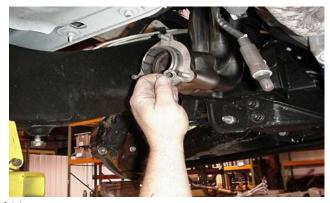
Install one spacer per stud. This prevents the gasket from being crushed beyond its intended yield point as the catalytic converters and "Y"-pipe are being tightened into position.
