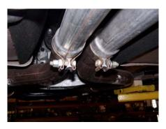
Spray the two down tube nuts on the left (driver) side with penetrating fluid and let soak. Remove the two nuts.
