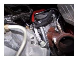
Begin removal of the left (driver) side cast manifold by removing the nuts holding the aluminum heat shield in place. The heat shield nuts are on each of 4 extended stud manifold bolts.
