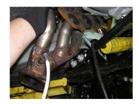
• Remove O2 sensors from manifolds
