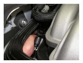
• Remove the outside nuts holding the cats to the manifolds on both sides
