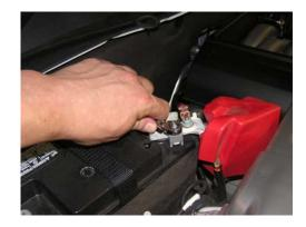
Remove wiring harness from battery tray before removing the battery tray
