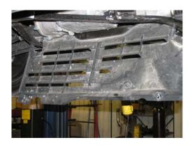
Next unbolt the plastic oil change access cover under the front of the engine. It is made to be loosened in the front and swings down and hangs in place.
