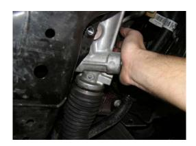
Reinstall the 2 rack and pinion bolts and torque to approximately 45 ft/lbs.
