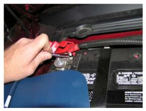
Removal of the battery and tray provides more room to get to the manifold bolts during a later step. Remove the battery cover and tie-down, the battery, and finally remove the battery tray by removing the 3 bolts holding the tray in position.
