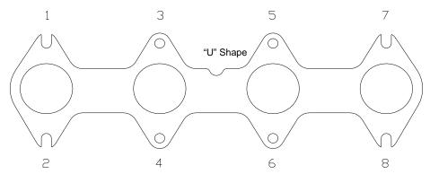
Use this torque chart for both the left and right header flanges.
