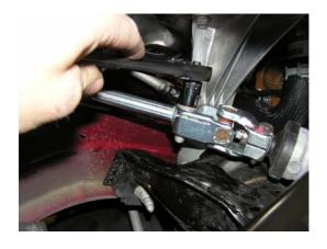
Install the steering shaft universal joint bolt and torque to 18 ft/lbs.
