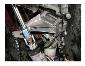
Attach the ground clamp to the front upper stud on the passenger side motor mount and securely tighten. The lower rear stud is either not used or holds a transmission cooling line clamp in the case of an automatic transmission.
