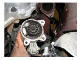
Remove the right hand motor mount by loosening and removing 2 bolts and 2 studs with nuts. The upper front stud is the mounting point for a ground cable. Remove the mount from the engine bay.
