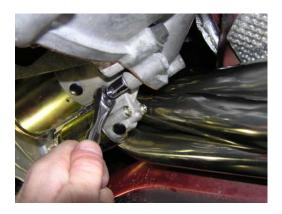
Re-install the starter (three bolts), attach the starter cables, and replace the protective red terminal cap.
