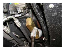
Support the front of the engine by placing a small block of wood or other suitable pad under the oil pan flange and the crankshaft pulley and raise the front of the engine 1 to 1 ½ inches.
