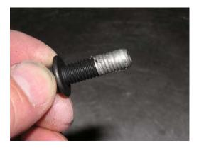
Prepare each of the 16 header bolts with a small amount of anti-seize on the thread surfaces.
