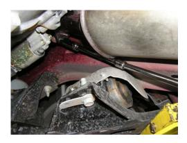
Page 7 of 20 GT Rev7  Remove the rear tailpipe couplers that were loosened in an earlier step by inserting the flat of a screwdriver under the spring tab and twisting to release while sliding the couplers rearward. Be sure to save these couplers, they will be reused during the installation of the new system.
