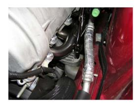
Install and tighten to specification the nuts securing the motor mounts to their respective frame mounts. Tighten these to approximately 46 ft/lbs.
