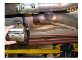
The "H"-pipe assembly should be completely free to remove at this point.
