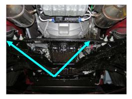
• Begin the under – vehicle procedures by loosening the band clamps securing the "H"-pipe to the tail pipes. Do not remove the clamps at this time.
