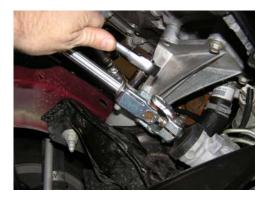
Loosen and remove the bolt holding the upper steering shaft section into the universal joint.
