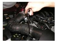
Check all work for completeness, bolts tightened, connectors connected, lines replaced and clamped etc. Check that no wires or lines are close to the headers where heat damage could occur or near moving parts where they could be pinched or cut. Check for misplaced tools and rags and check for oil leaks etc.
