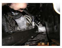
Remove the 2 bolts holding the steering rack and pinion into cross-member.  Slide the rack and pinion forward in the car enough to allow the upper steering shaft to slip out of the universal joint. Lay the steering shaft out of the way on top of the frame rail. Caution: Do not allow the steering wheel to rotate while the steering column intermediate shaft is disconnected – damage to the clock spring can result. If this occurs the clock spring must be removed and re-centered.
