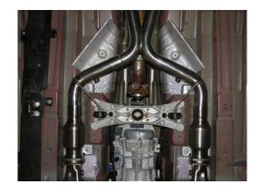
• Reinstall the saved OEM band clamps over the stock tailpipe, raise the rear of the x-pipe assembly and slide the clamps over the x-pipe outlets. Make sure that the joint where the x-pipe outlets and the tails are joined, that the tubes are butted up as close as possible to one another by moving the x-pipe assembly back to meet the tailpipes.
