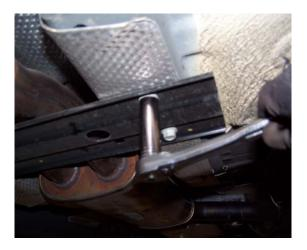
Unbolt factory exhaust at the rear of the car at the mufflers and remove exhaust from front and rear rubber hangers and remove from vehicle
