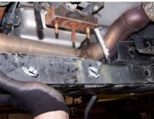
• Remove the front rubber muffler hanger
