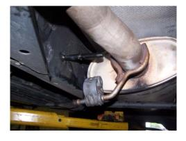
Next, loosen and remove the three (3) nuts on both the left (driver) side and right (passenger) side down tubes and remove y-pipe. Penetrating fluid may be helpful.
