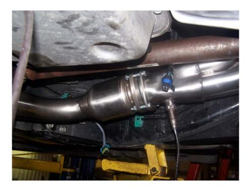
With the cross over tube in place, slip the 2 ½" stainless band clamp over the outlet end of the cross over tube and connect to the y-pipe.
