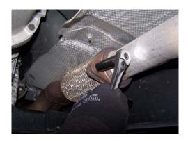
Remove the heat shields from the floor board and the left side frame rail.
