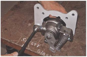
5. Insert the brake pads in the caliper and install the caliper brackets as shown using the supplied Allen-head slider bolts.
