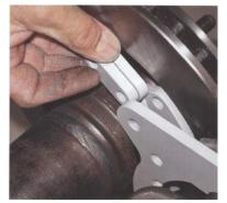
6. Test fit the caliper on the rotor, making sure the bleed screw is facing up. Your brake kit comes with bracket spacers in two different thicknesses. Determine the number and thickness of spacers required to properly position the caliper in relation to the rotor.
