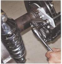
9. Install caliper on bracket using supplied Allen-head slider bolts.
