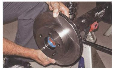
4. Install the rotor over the axle studs and temporarily secure using two hand-tightened lug nuts.
