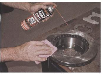
3. Make sure to use a quality brake cleaner and rag to clean the anti-corrosion coating off your brake rotors before installing them. This coating can contaminate brake pads.
